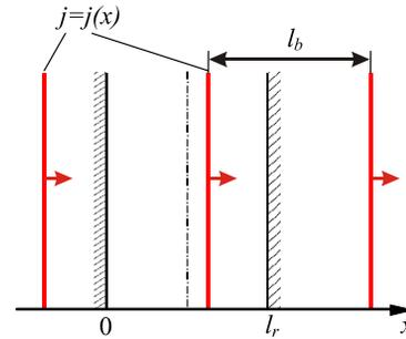
Figure 2: One-dimensional model of resonator with passing sequence of bunches.
