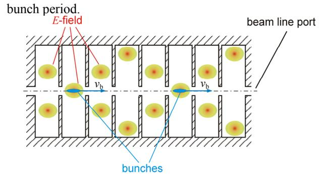
Figure 1: Acceleration of moving periodic bunches by cavities operated with a superposition of synchronized eigenmodes.
