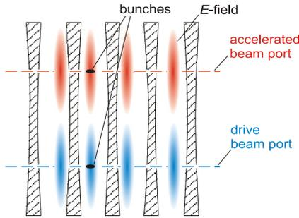
Figure 3: Two-beam accelerating structure based on two-mirror cavities.
