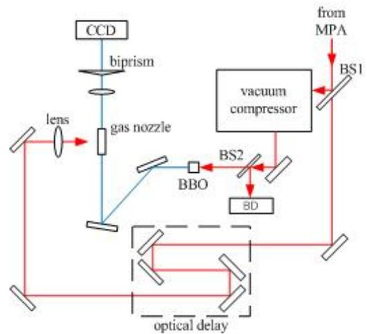
Figure 3: Schematic diagram of the experiment.
