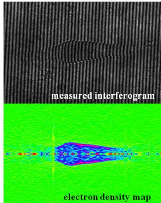
Figure 4: Electron density structure. Upper panel shows the measured interferogram and lower panel shows density map. Laser direction is from right to left.
