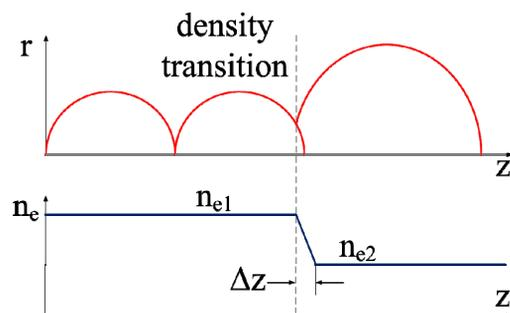
Figure 1.: Schematic diagram of the electron injection using density transition.
