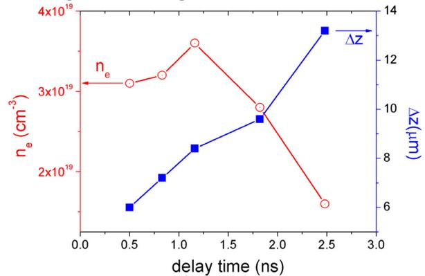
Figure 6: The measured density structure at different time. Open circle show the peak density at the boundary of the plasma. Closed square line shows the density transition length.
