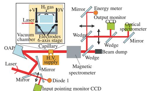
Figure 1: Experimental setup. The detailed description of the electron spectrometer can be found in Ref. [8].
