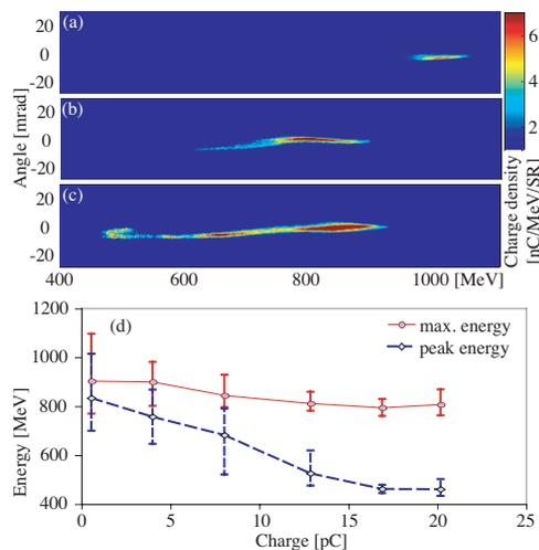
Figure 2: (a)-(c) Representative single shot e-beam spectra, (d) the peak energy and maximum energy versus charge for the 33 mm long, 300  $\mu\text{m}$  diameter capillary. (The plasma density was  $\sim 5.3 \times 10^{18} \text{ cm}^{-3}$ , the laser was 1.5 J–46 fs, the applied voltage was 18 kV, and the discharge delay was  $\sim 580$  ns.)
