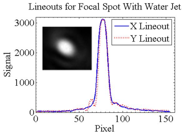
Figure 5: Near field image of the mode of TREX laser reflected from water jet at  $\approx 50$  torr pressure.
