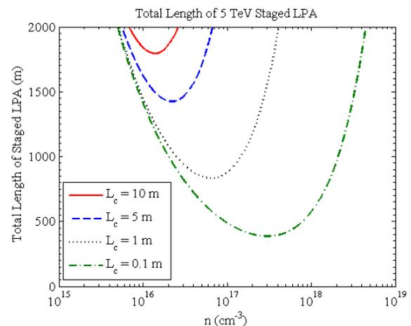
Figure 2: Main single-linac length versus plasma density  $n_0$  for several laser in-coupling distances  $L_c$ ,  $E_b = 5 \text{ TeV}$  and  $a_0 = 1.5$  [6]
