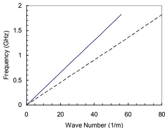
Figure 2: Dispersion characteristics obtained from Eq. (13) for the parameters listed in Table 1. The solid curve is for the fast-space-charge waves, whereas the dashed curve is for the slow-space-charge waves.
