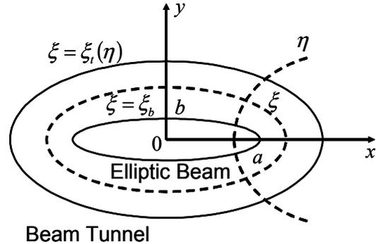
Figure 1: Cross section of a relativistic elliptic electron beam system.
