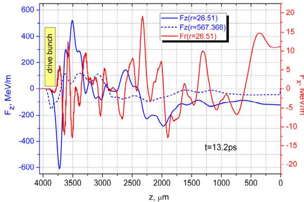
Figure 5: Axial (blue solid line) and transverse (red line) forces acting upon accelerated electrons versus  $z$ , the latter at  $r = 26.5$   $\mu\text{m}$ . Dashed blue line shows the force acting upon electrons at the center of the drive channel, at  $r = 567.4$   $\mu\text{m}$ . Time of observation is  $t = 13.2$  ps.
