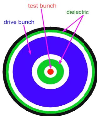
Figure 1: Cross-section of a coaxial dielectric accelerator structure (CDS). Dielectric tubes are green, drive bunch is blue; test bunch is red, and black outer shell is metal.
