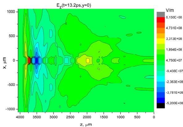
Figure 4: Map of axial wakefield in CDS at time  $t = 13.2$  ps after injection. Drive bunch is at the far left.
