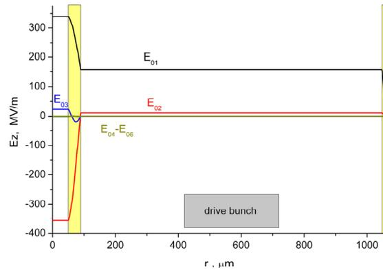
Figure 2: Transverse profiles  $E_z(r)$  for the first six TM-modes, with the  $E_{02}$  operating mode. Locations of the two dielectric shells are highlighted in yellow.
