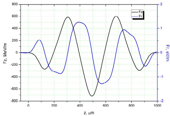
Figure 3: Axial profiles of composite longitudinal force (black line) and the composite transverse force (blue line), the latter at the distance of 25  $\mu\text{m}$  from center of the accelerating channel. The drive bunch moves from right to left and its center is located at  $z = 0$ .
