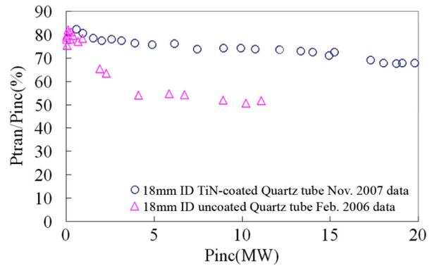
Figure 3: RF transmission percent versus incident power for 18-mm ID quartz tubes, uncoated and with TiN coating.
