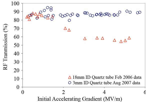
Figure 2: RF transmission percent versus accelerating gradient for 3-mm and 18-mm ID quartz tubes.
