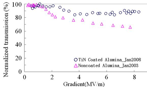
Figure 4: Normalized RF transmission percent for 1-cm ID alumina tubes, uncoated and with TiN coating.
