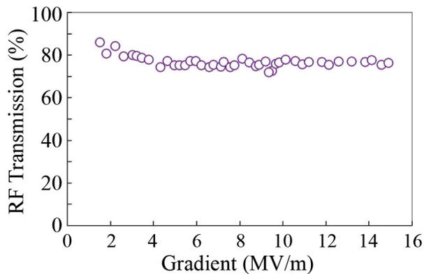
Figure 5: RF power transmission percent versus incident power for clamped quartz structure.
