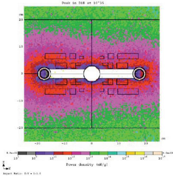
Figure 2: Heating calculation for LHC circulating beam in open midplane dipoles by N. Mokhov
