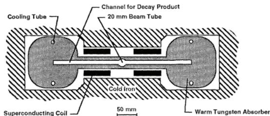
Figure 1: Concept of the first "open midplane" dipole
