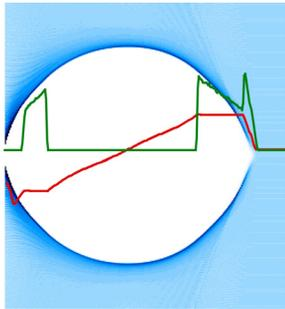
Figure 1: The longitudinal profiles (green curve) of the drive and main beams and the longitudinal wakefield (red curve) produced by these beams. The blue and white background are plasma and the ion channel, respectively.
