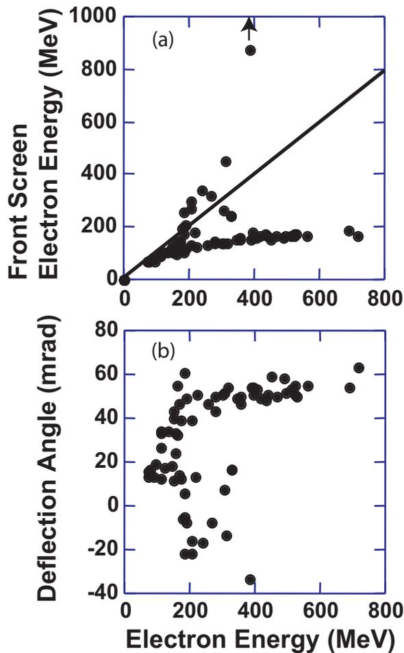
Figure 2: a) The energy of each of our electron beams is measured first using both image plates and then again with just the front image plate. The solid line divides electron beams with positive (below the line) and negative (above the line) deflection angles. b) The deflection angles for all electron beams are shown; there is no apparent correlation to beam energy.
