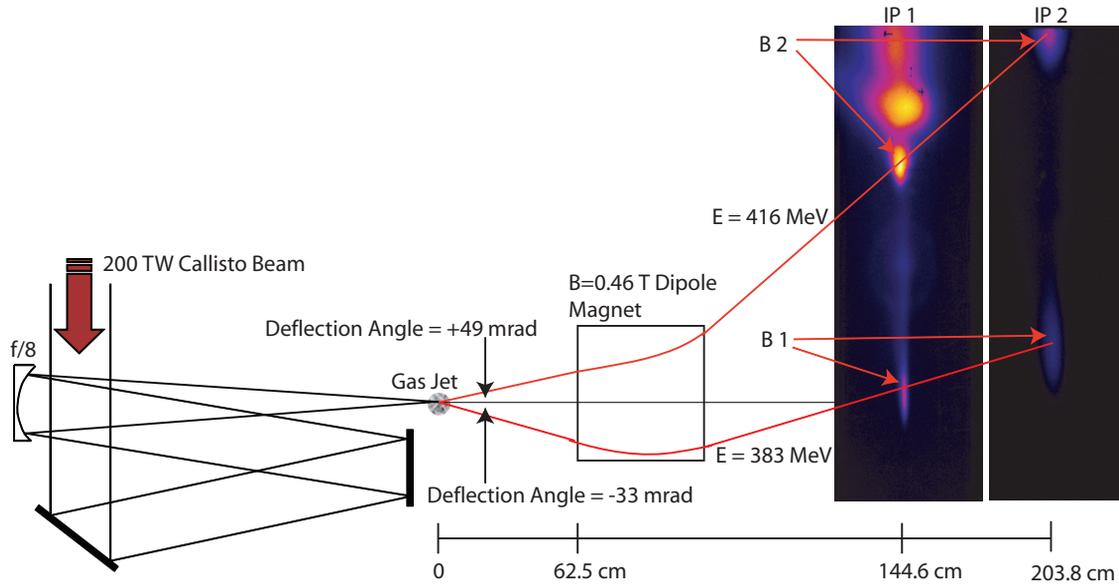
Figure 1: The 200 TW Callisto laser is focused by an f/8 off-axis parabola to a vacuum spot size of 18 microns (FWHM) at the leading edge of a gas jet. The jet delivers He gas at neutral densities of  $1 \times 10^{18}$ - $1 \times 10^{19}$   $\text{cm}^{-3}$ . A dipole magnet is placed after the jet, followed by two image plates. The displayed trajectories through the magnet correspond to the features labeled B1 and B2 on the image plates.
