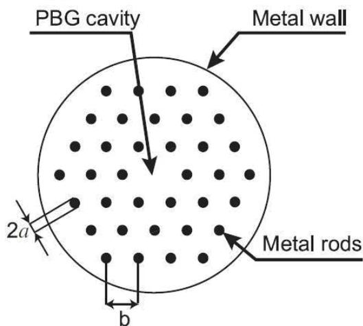
Figure 1: The geometry of a PBG resonator formed by removing a single rod in a triangular array.
