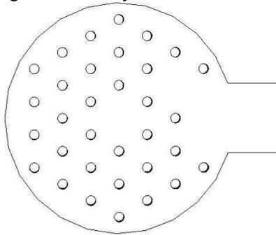
Figure 4: Coupling scheme for the PBG resonator in Fig. 5.
