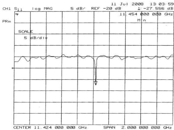
Figure 3: Cold test measurement of the PBG cavity.
