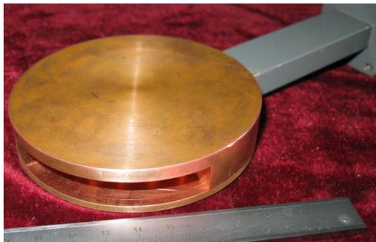
Figure 5: PBG resonator with a WR90 waveguide fabricated.
