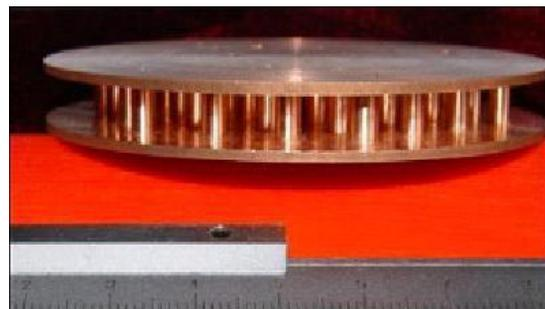
Figure 2: PBG cavity built for cold test.
