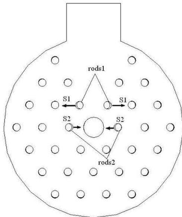
Figure 7: The coupling scheme of the Traveling wave structure proposed by Tsinghua University.
