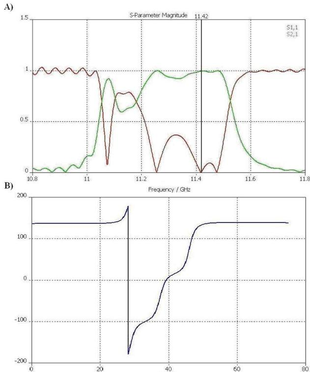
Figure 8: Simulation results of the 4-cell PBG accelerator: A) S parameters; B) Phase shift of electric field along axis
