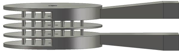
Figure 9: 3D model of the 4-cell PBG accelerator.
