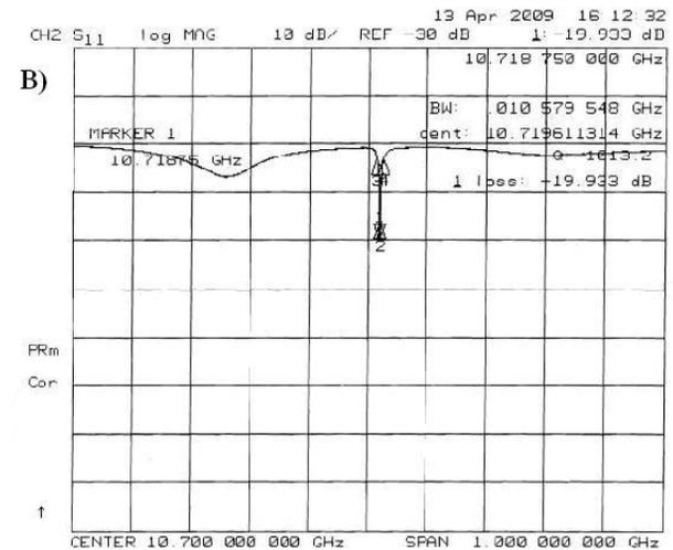
Figure 6: A) Numerical simulation result of the PBG resonator in Fig.5), B)Cold test measurement of the resonator.
