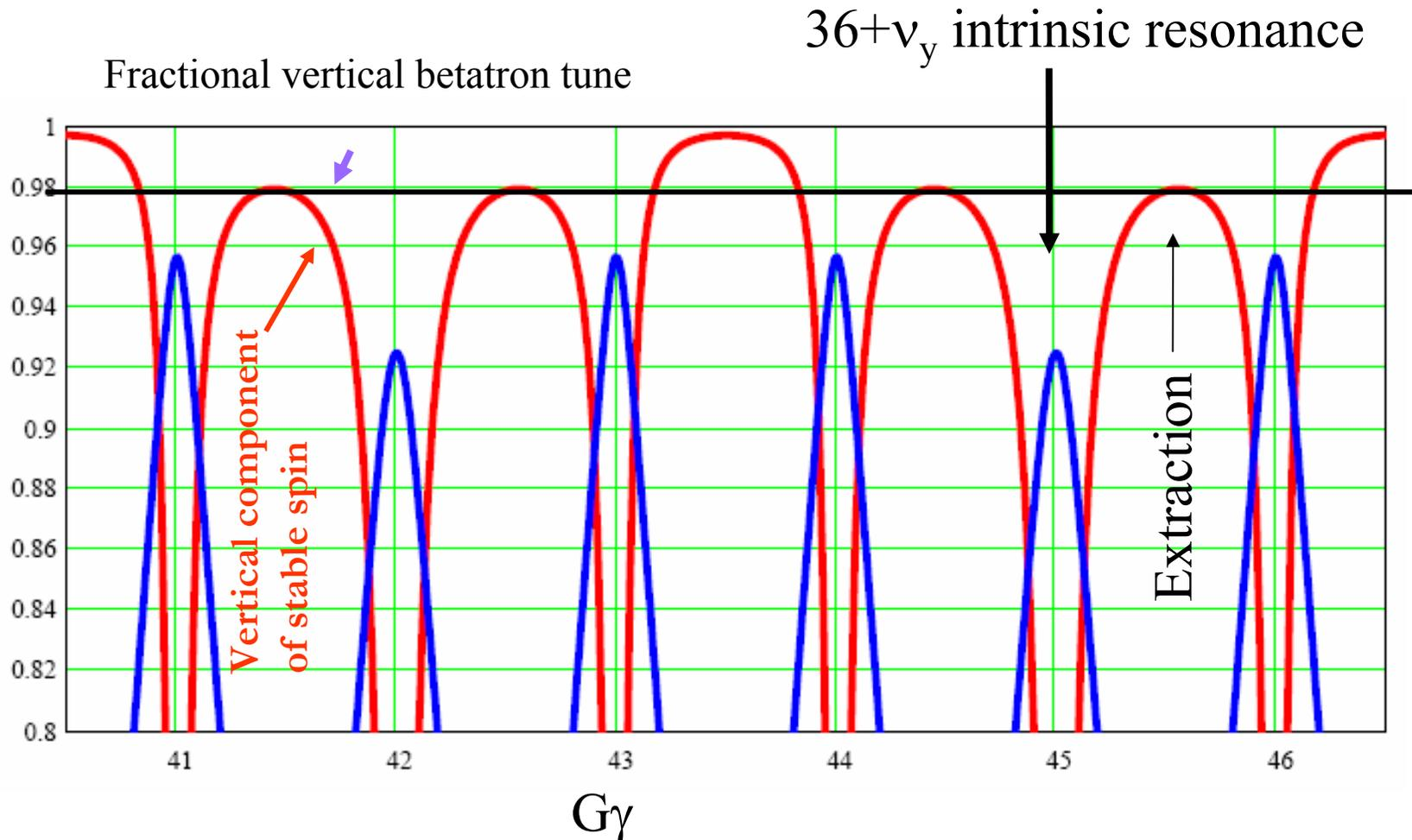
Spin tune gap modulation of the period of 3 units of  $G\gamma$ :
