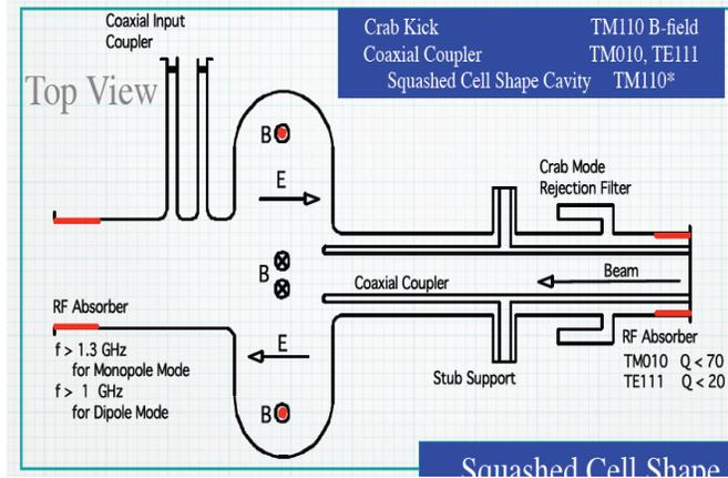
KEKB cavity: angle: 11 mrad,  $V_{\text{kick}}$ : 1.4 MV
