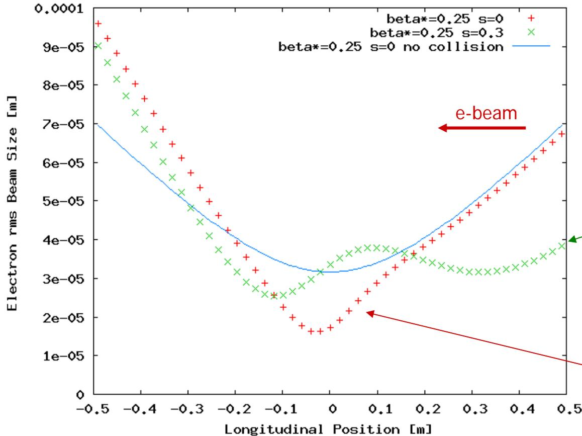
Proper selection of the IP  $\beta$  and  $\beta$ -waist is important to minimize the proton beam-beam parameter
