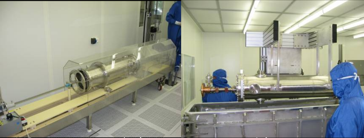
HPR rinsing and clean room assembling in the IPN Orsay SupraTech clean room
