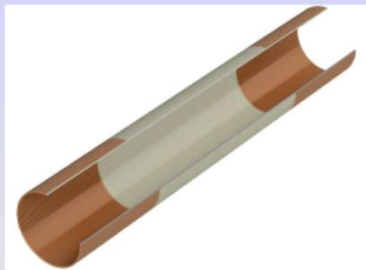
A pipe with a high wall conductivity (perfect conductor) has a short resistive insert of length  $L_i$ .
