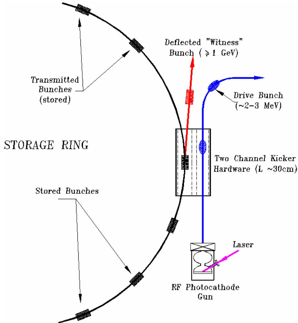
A rectangular two-beam dielectric wakefield accelerator (DWFA) is under study in a collaboration between Omega-P, Yale, Columbia, and ANL. Due to asymmetry, this structure will deflect a test bunch moving in the narrow channel, due to wake fields set up by drive bunches in the broad channel.
