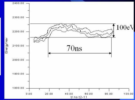
Time-resolved beam emittance measurement Cerenkov Radiation with streak camera
