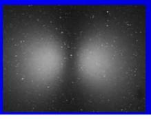
Distribution of OTR at different divergence angles of beam at energy of 20MeV
