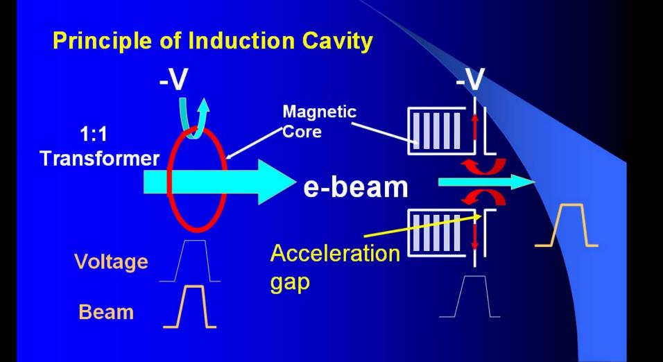
**Principle of Linear Induction Accelerator**
