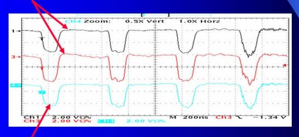
Beam pulses(CH3)~2 kA
