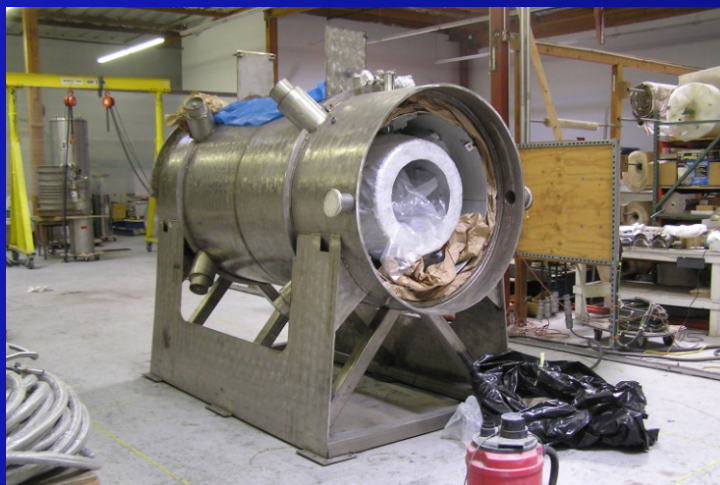
Spectrometer Solenoid being assembled
