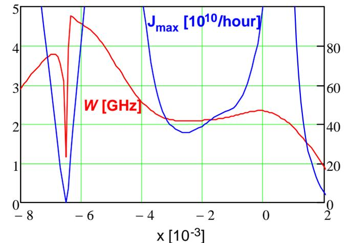
*Dependences on momentum for the cooling force, its phase, effective bandwidth and Van der Meer flux*
