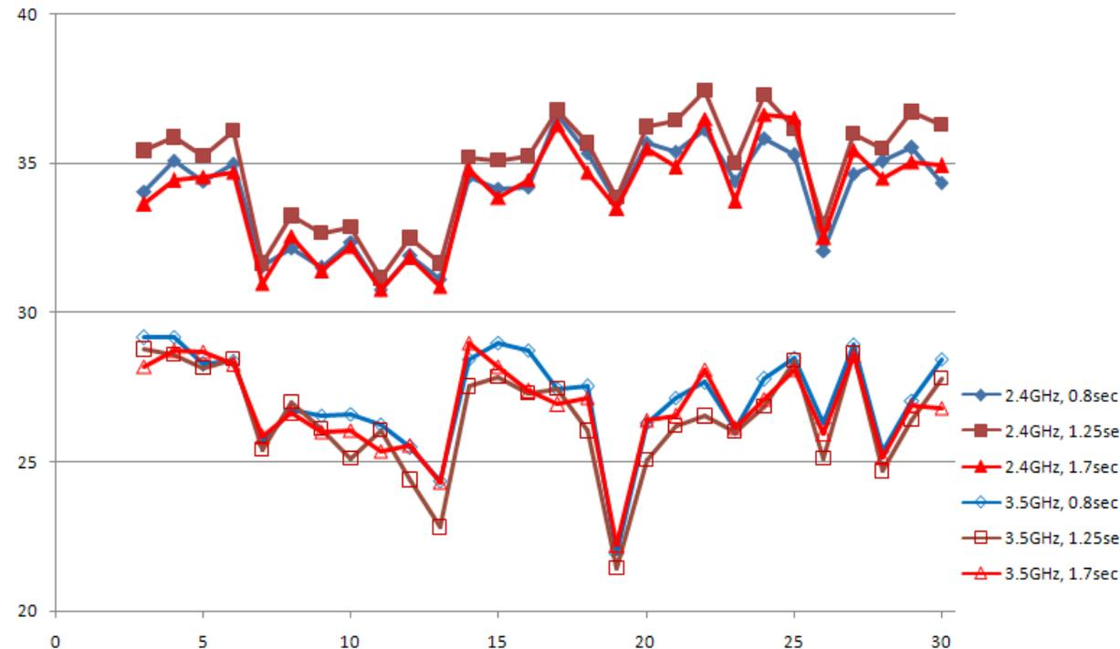
*Notch depth at different times in cycle for 2.4 and 3.5 GHz*
