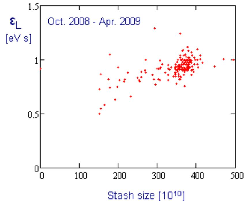
*Dependence of longitudinal emittance in MI, 8 GeV, on stash size*
