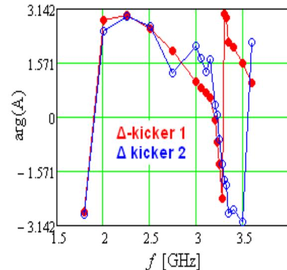
*Amplitudes of  $\Delta$ -kickers required for compensation of dipole part of transverse kicks*
