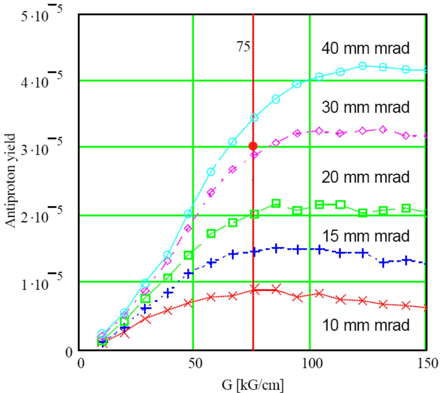
*Dependence of Computed Antiproton yield on Debuncher acceptance and lithium lens gradient*
