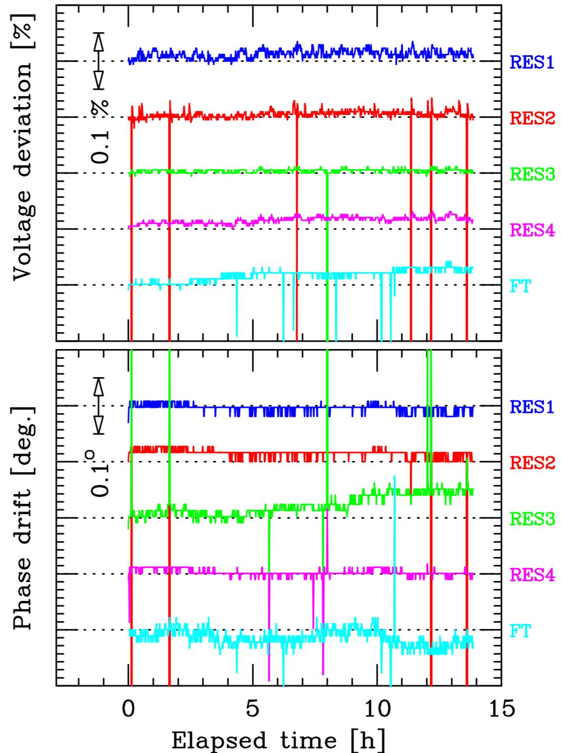
$\Delta V/V \sim 0.01\%$   $\Delta \psi \sim \pm 0.1^\circ$  RF
