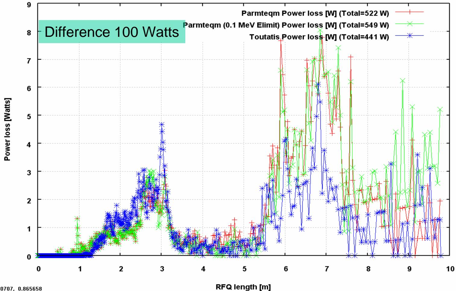
Plot of RFQ Power Loss as function of RFQ length, The toutatis runs are made with 1'000'000 macroparticles.
