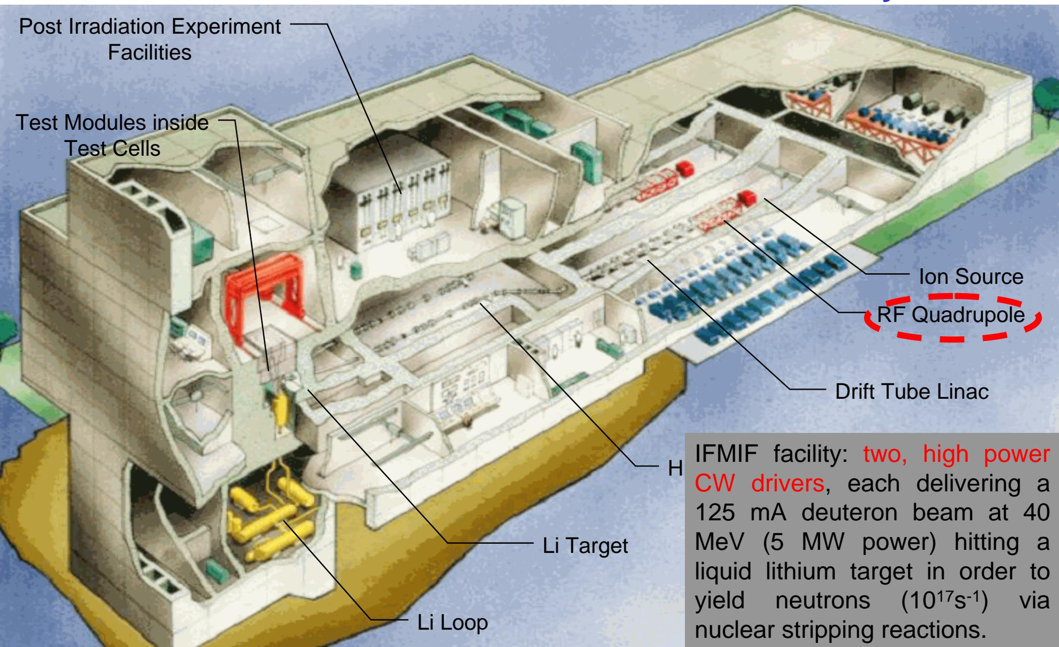
IFMIF facility: **two, high power CW drivers**, each delivering a 125 mA deuteron beam at 40 MeV (5 MW power) hitting a liquid lithium target in order to yield neutrons ( $10^{17}\text{s}^{-1}$ ) via nuclear stripping reactions.
