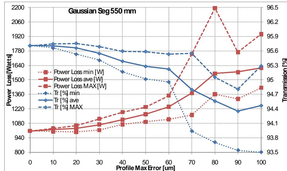
Transmission and Power loss due to the segmentations applied with gaussian and waterbag input beam distribution. (TOUTATIS)
