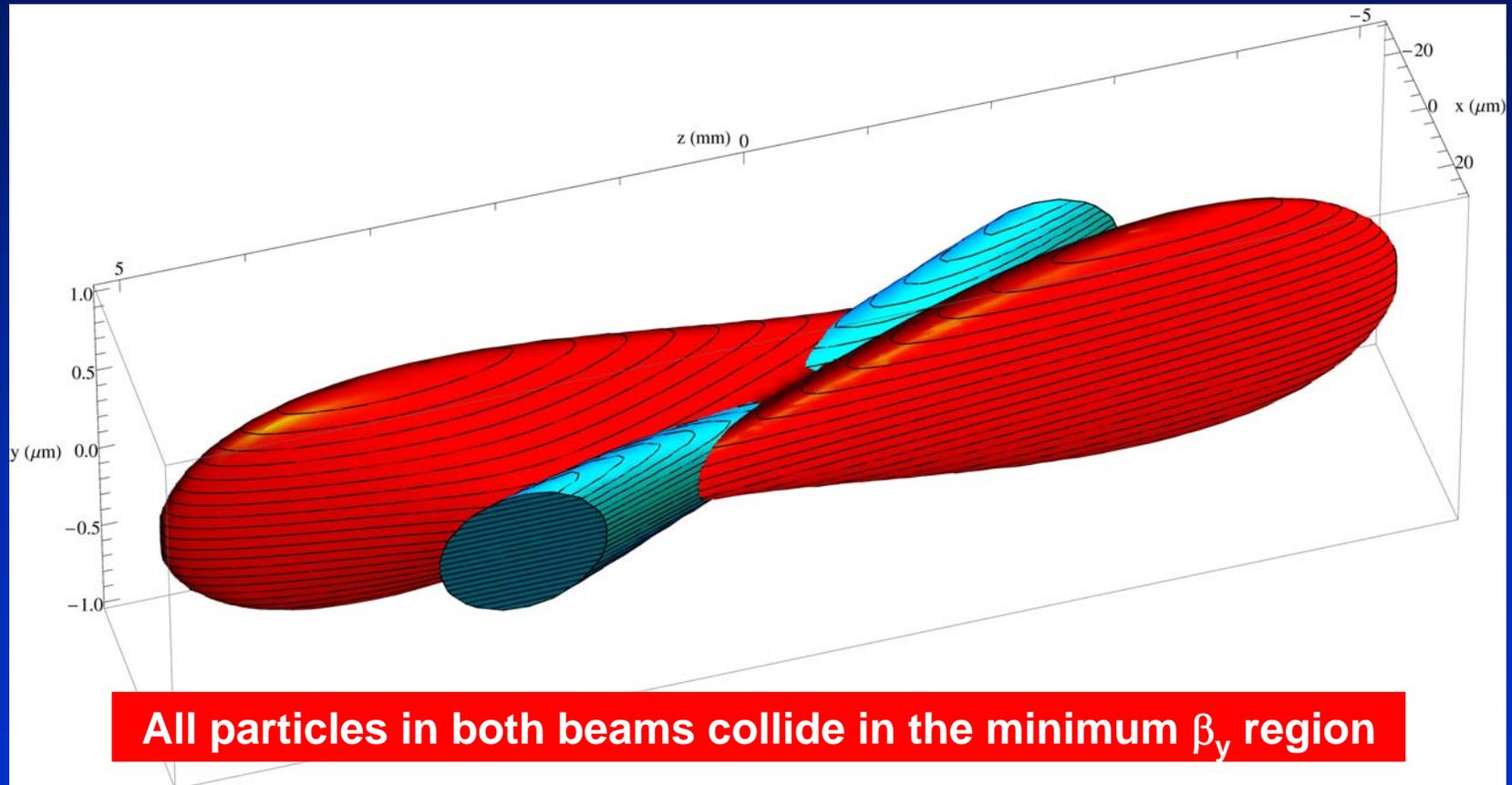
Crab sextupoles ON: Waist moves parallel to the axis of other beam: maximum particle density in the overlap between bunches
