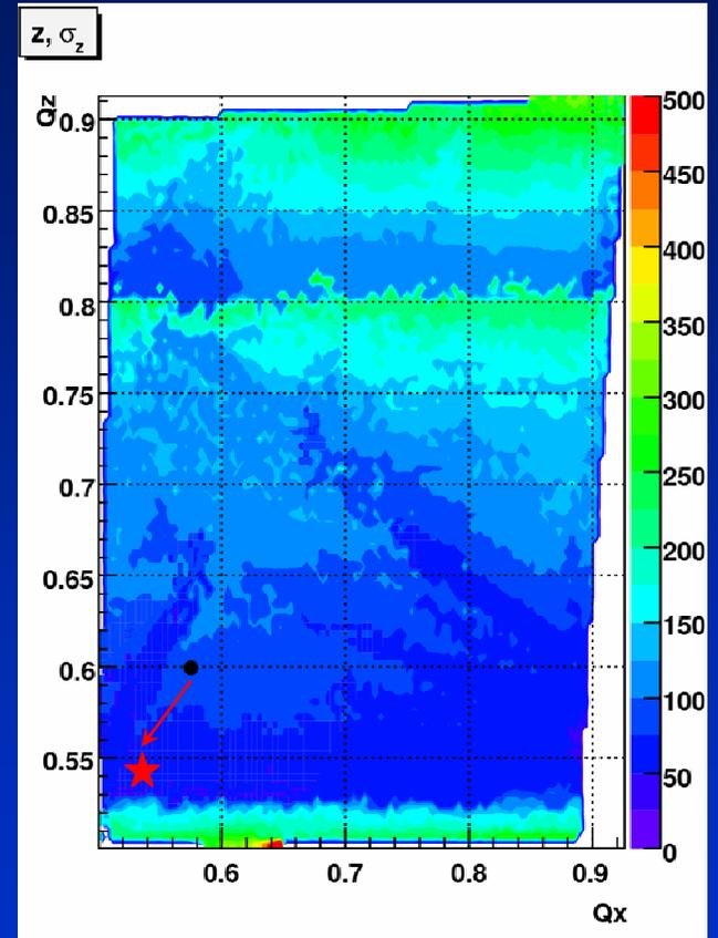
Beam-beam simulations taking into account nonlinear lattice elements have indicated that further dynamic aperture optimization is required in order to increase the beam lifetime (in progress)
