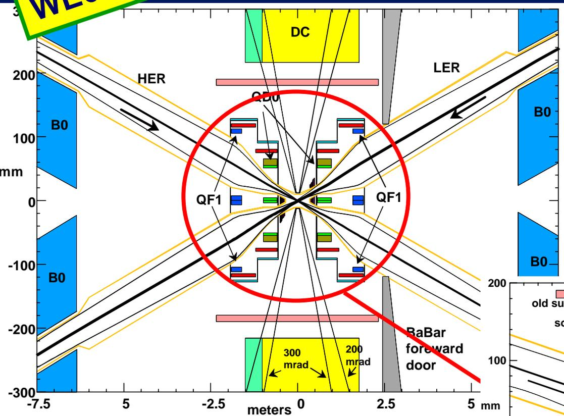
With a larger crossing angle (60 mrad total) beams are far enough apart at 0.35 m from the IP to have enough space to install a PM, in front of QD0, for LER which needs more focusing
