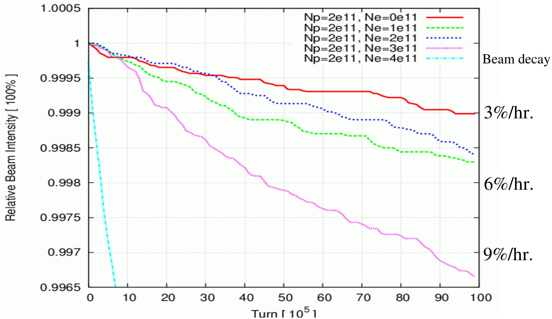
From simulation, stronger than HBBC has negative effect on beam lifetime.
