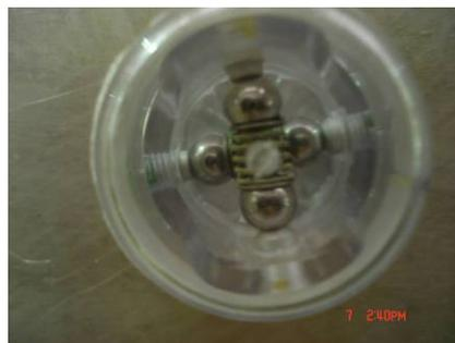
**Shock detectors are intact; klystron is safely received**
