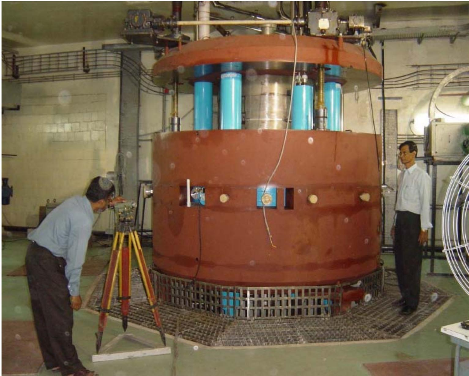
**Magnet assembly with pole cap in lifted position - maximum lifting height of upper pole cap is 1143 mm.**
