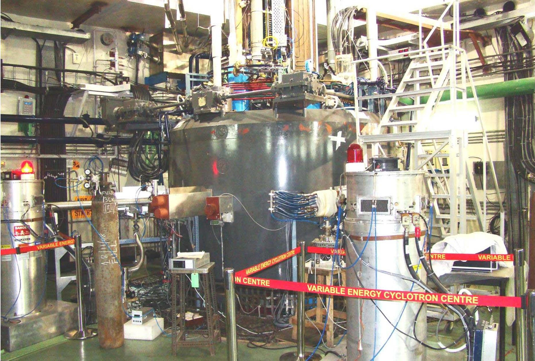
**VIEW OF THE SUPERCONDUCTING CYCLOTRON IN VAULT**
