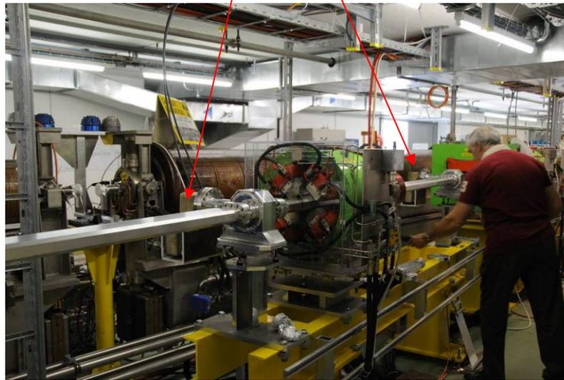
**Circular Profile Vacuum Chambers installed**
