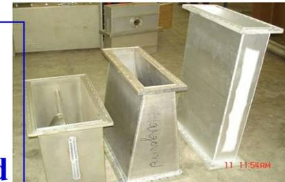
**Klystron handling equipment & WR 2300 waveguide components designed and developed at RRCAT**
