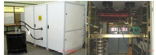
Figure 4 left: resistive load in oil tank (@110kv) connected to modulator; right: bouncer circuit elements pictures at RRCAT
