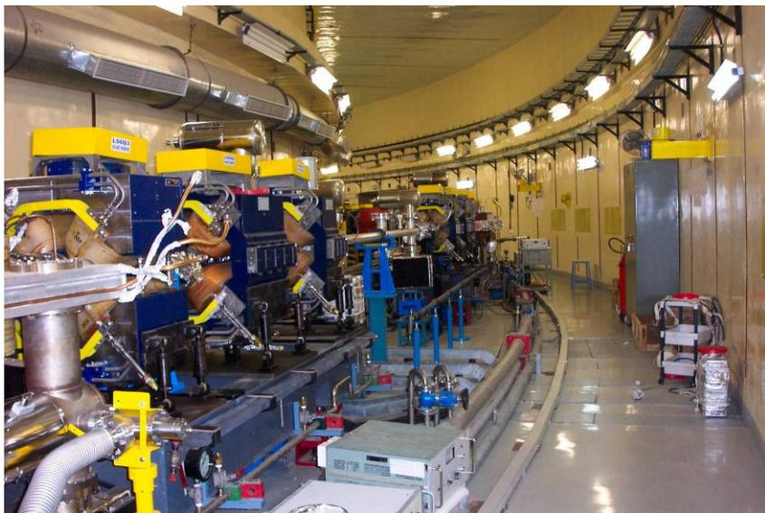
RF Cavities installed in Indus-2 Ring
