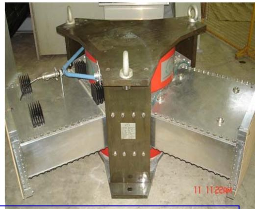
**LEP Klystron and circulator received from CERN being integrated with test stand at RRCAT**
