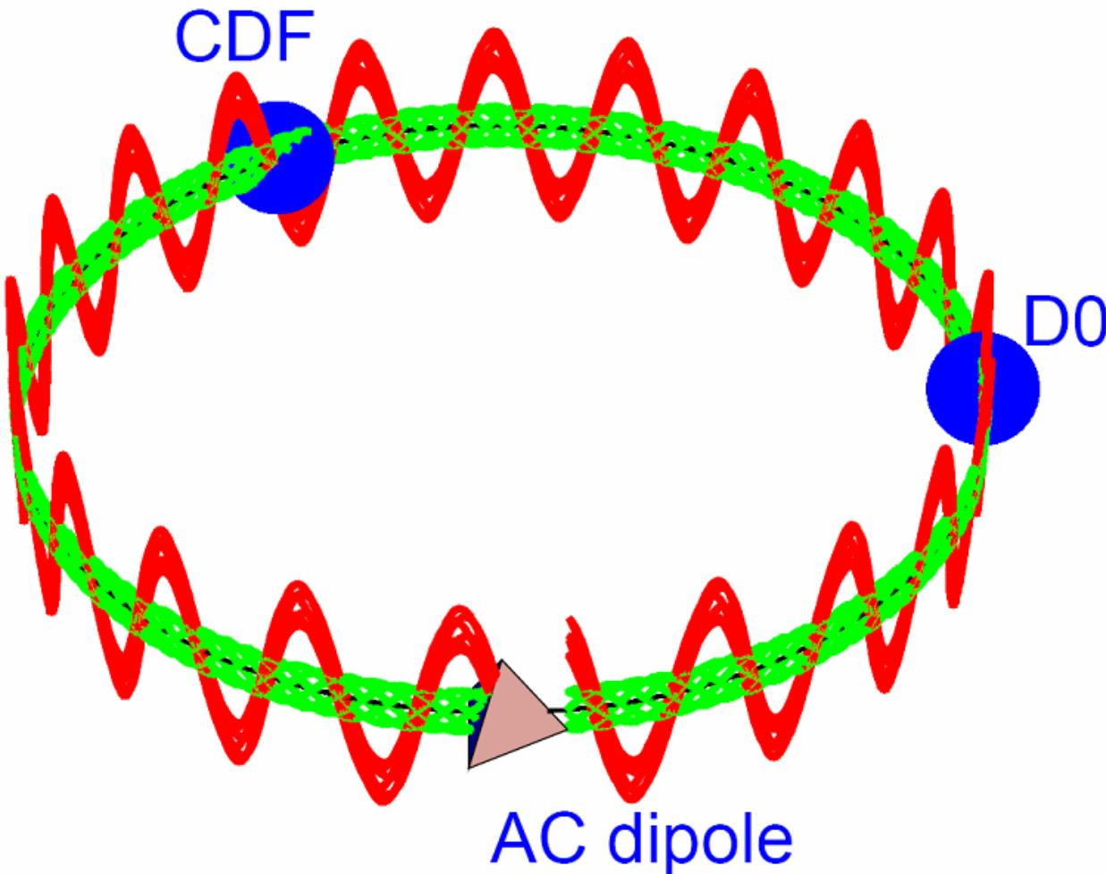
An AC dipole excites the beam with its sinusoidally oscillating dipole field ( $f_{\text{ac dipole}} \sim f_{\text{betatron}}$ ).
