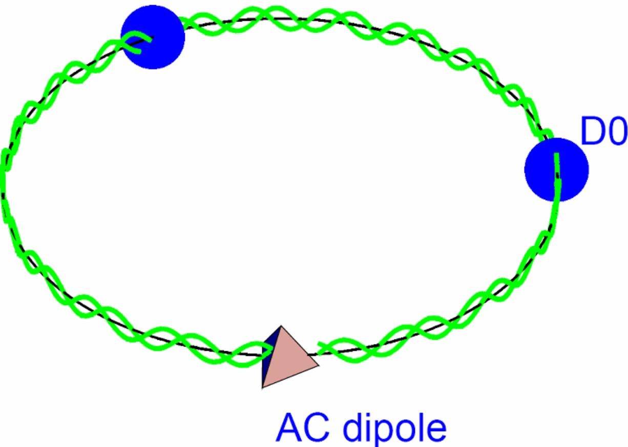
An AC dipole excites the beam with its sinusoidally oscillating dipole field ( $f_{\text{ac dipole}} \sim f_{\text{betatron}}$ ).
