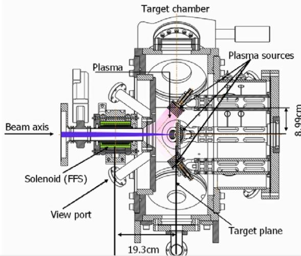
Plasma density  $> 10^{13} / \text{cm}^3$  after modifications to FCAPS: straight filters, 2  $\rightarrow$  4 sources, increased  $I_{\text{discharge}}$
