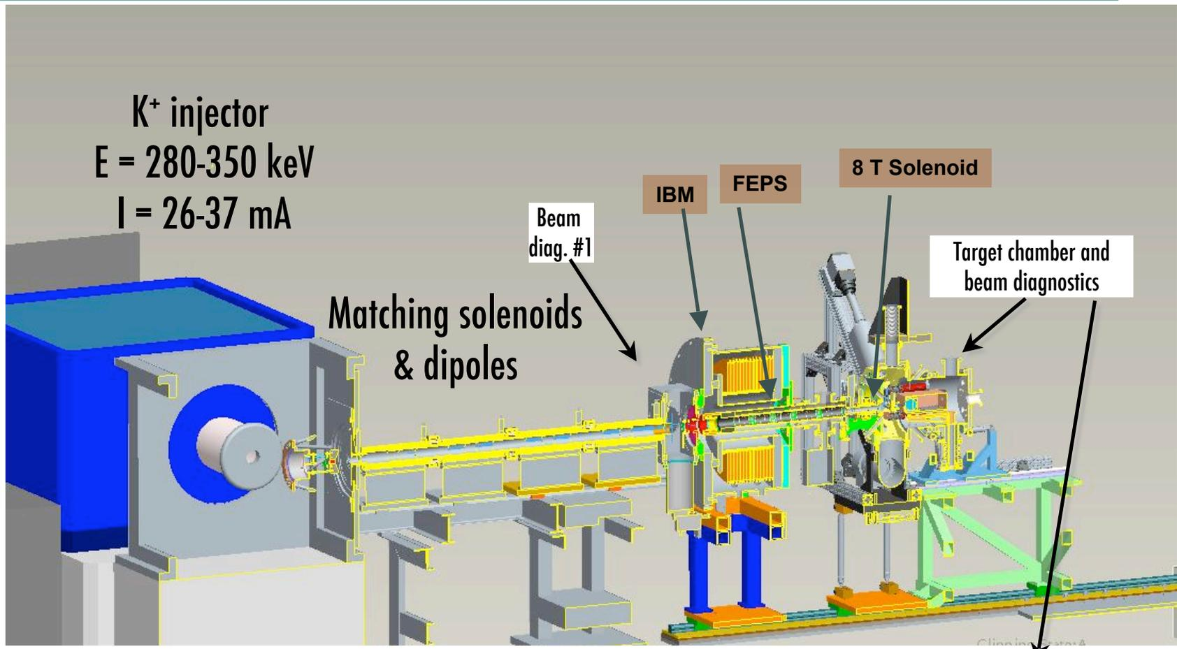
**Objectives:** Preservation of low emittance, plasma column with  $n_p > n_b$ , ( $\epsilon_{ni} = 0.07 \text{ mm-mrad}$ ,  $n_{b\text{-init}} \approx 10^9 / \text{cm}^3$ ,  $n_{b\text{max}} \approx 10^{12} / \text{cm}^3$  now, later,  $\approx 10^{13} / \text{cm}^3$ )
