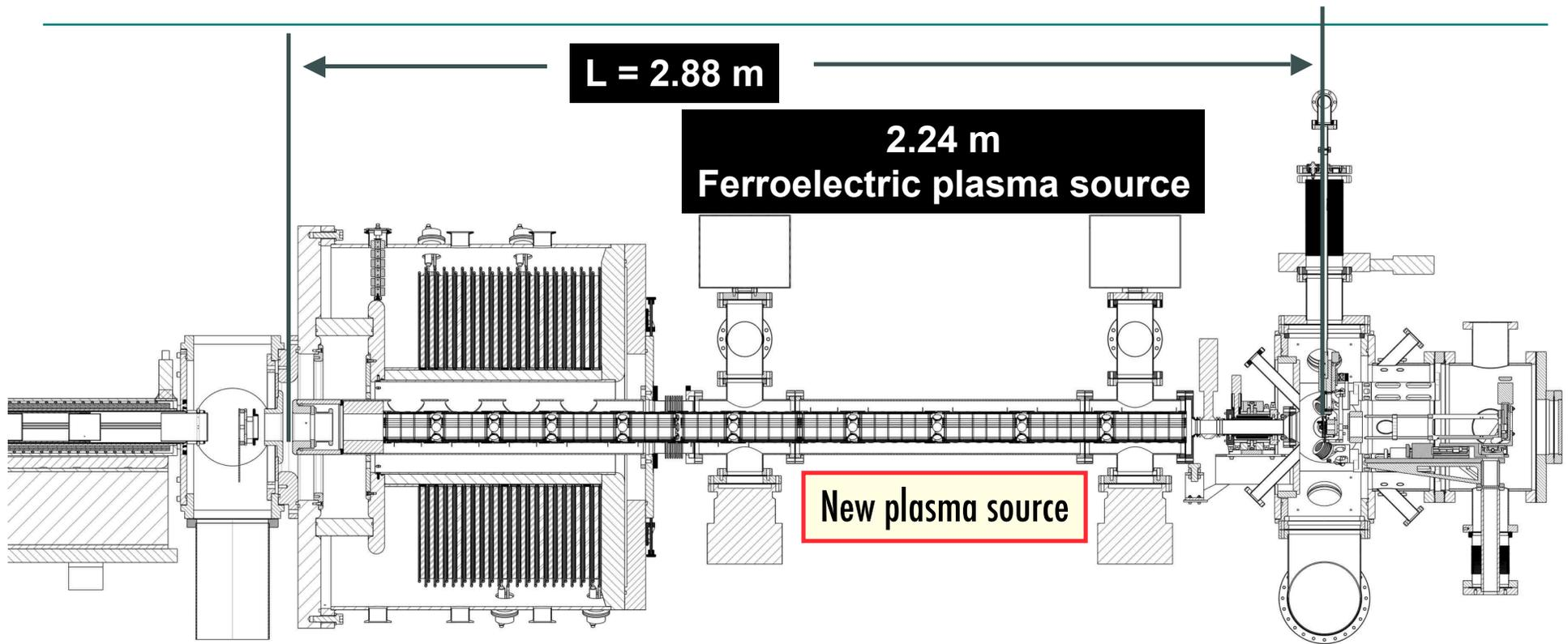
~2x longer drift compression section ( $L=2.88 \text{ m}$ ), Uses additional volt-seconds for a longer ramp and to limit  $\Delta V_{\text{peak}}$  & chromatic effects
