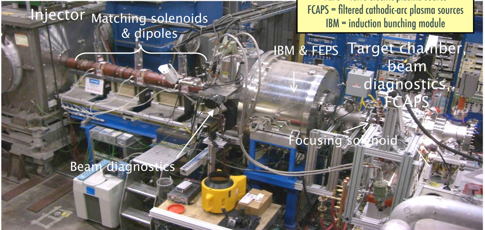
New: steering dipoles, focusing solenoid (8T), target chamber, more diagnostics, upgraded plasma sources
