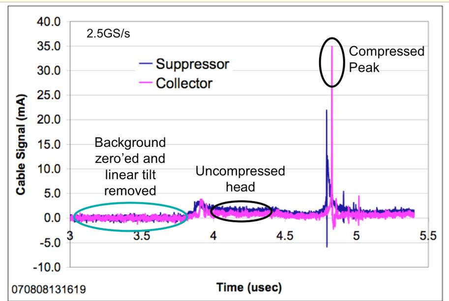
$$I_{\text{beam}} = I_{\text{collector}} \times (\text{transparency})^{-1}$$
