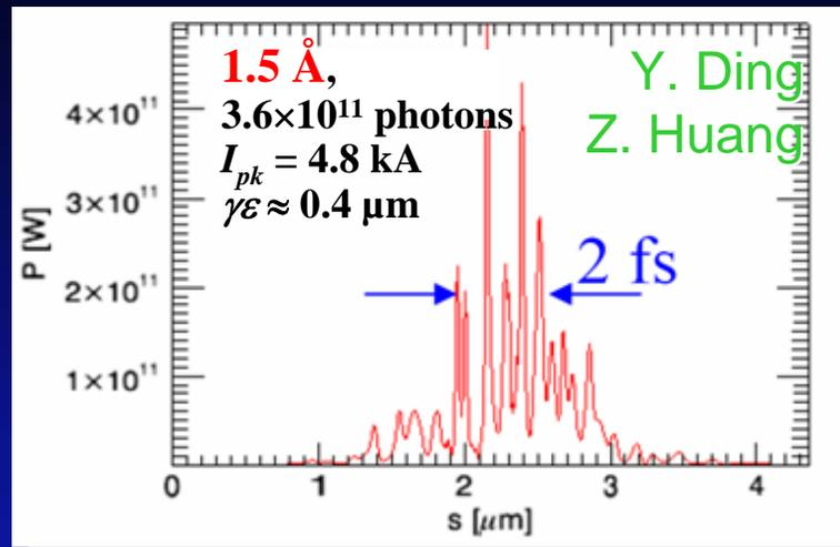
Simulation at 1.5 Å based on measured injector & linac beam & *Elegant* tracking, with CSR, at 20 pC.
