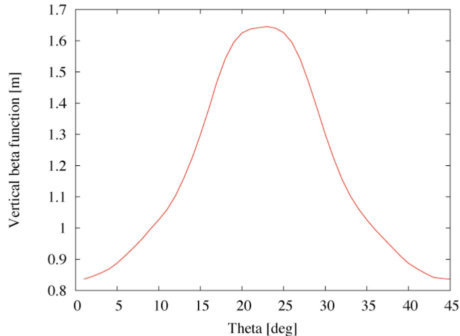
Vertical beta function@target  $\sim 0.83$  [m]
