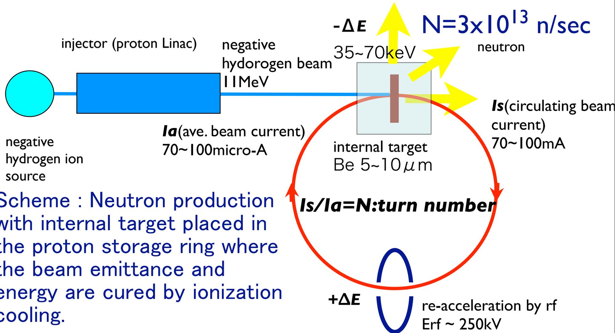
Scheme : Neutron production with internal target placed in the proton storage ring where the beam emittance and energy are cured by ionization cooling.
