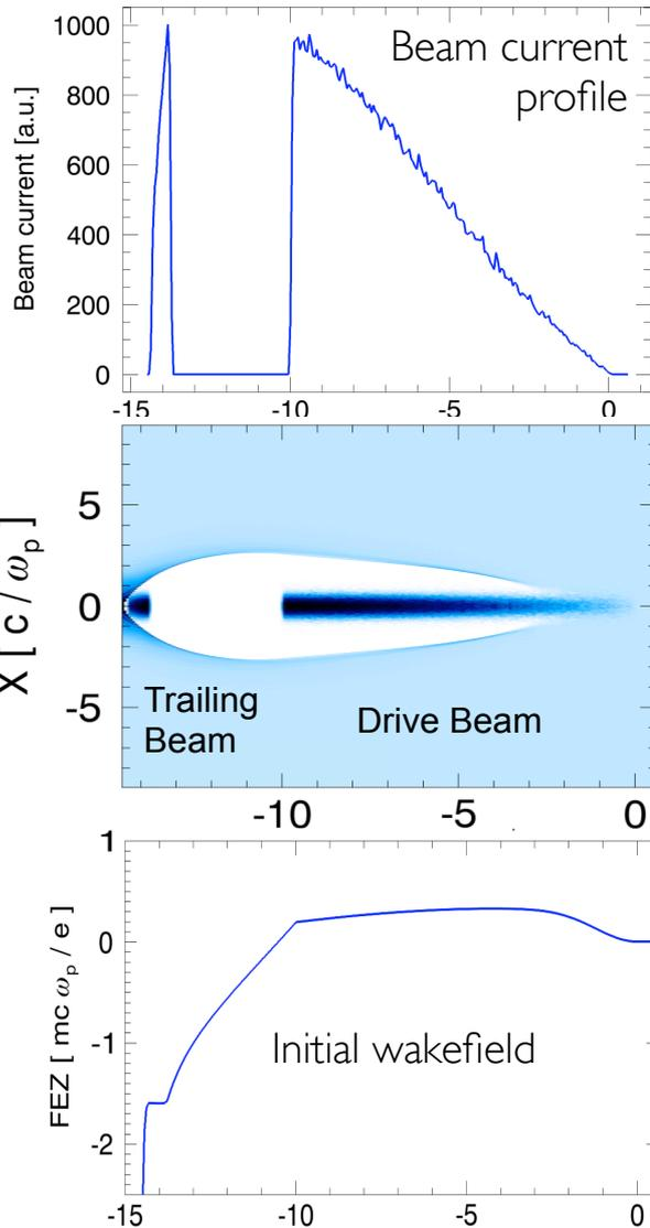
Higher efficiencies possible with non-gaussian bunch profiles
