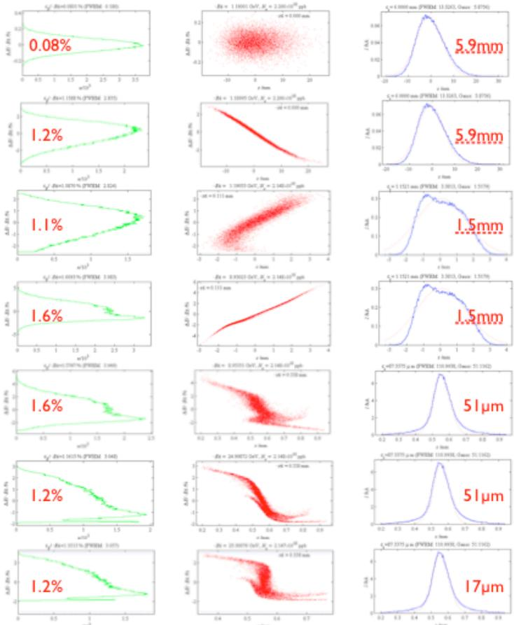
**Exploit Position-Time Correlation on e- bunch to create separate drive and witness bunch**
