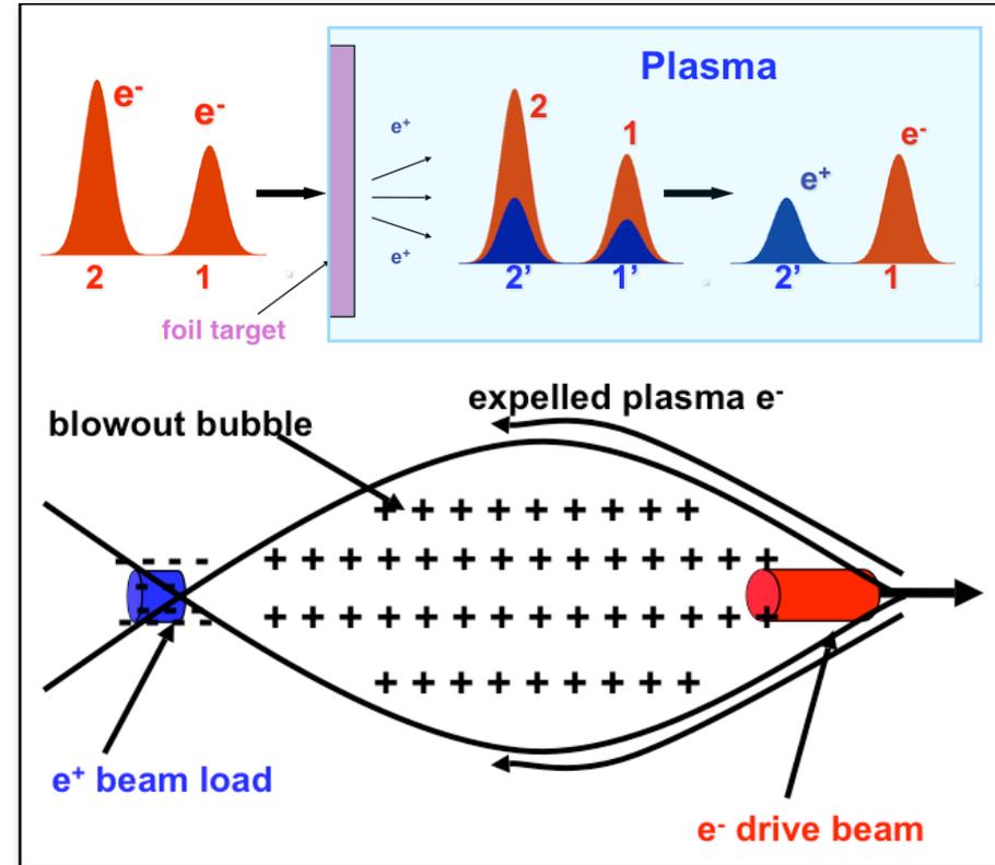
Generating closely-spaced mixed-species bunches is simplified by creating the positrons in the plasma
