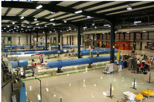
F422- Dipole assembly in cryostat (cryostating) learning curve - SMA18
