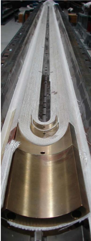
Scale up of TQ design from 1 m to 3.6 m length
