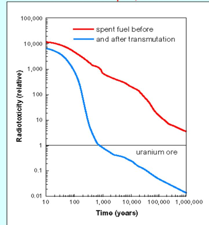
**Fig. 1** – Ingestion radio-toxicity of 1 ton of spent nuclear fuel. With a separation efficiency of 99.9% of the long-lived by-products from the waste, followed by transmutation, reference radio-toxicity levels can be reached within 700 years
