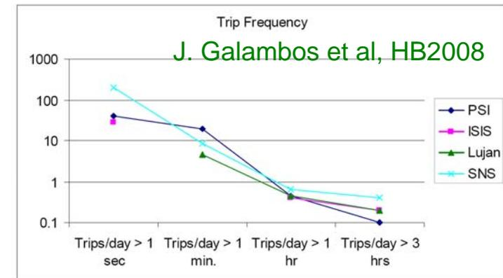
Figure 6. Trip frequency vs. trip duration for high power proton accelerators.
