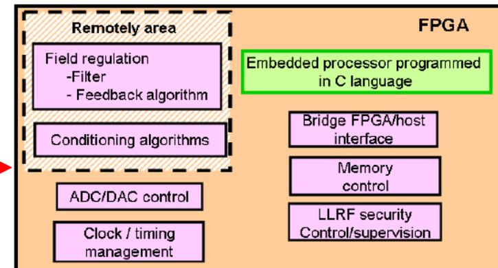
Figure 12: Internal architecture of FPGA
