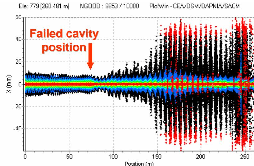
Figure 12 : Transverse beam distribution at 220  $\mu$ s, in red are plotted the losses
