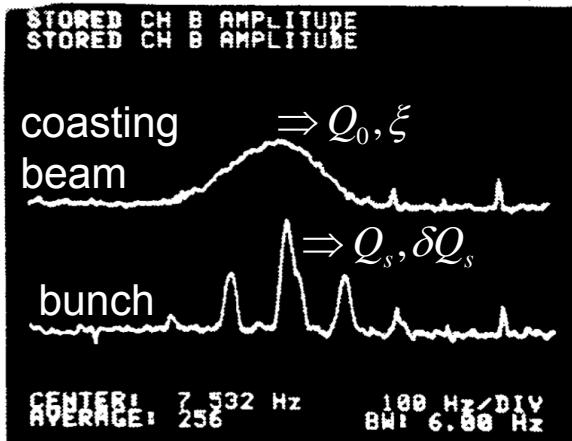
**Sum signal**  $U_\Sigma$ : beam current fluctuations  $\Delta I$
