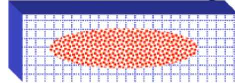
Solve Poisson equation on a rectangular domain with open BC
