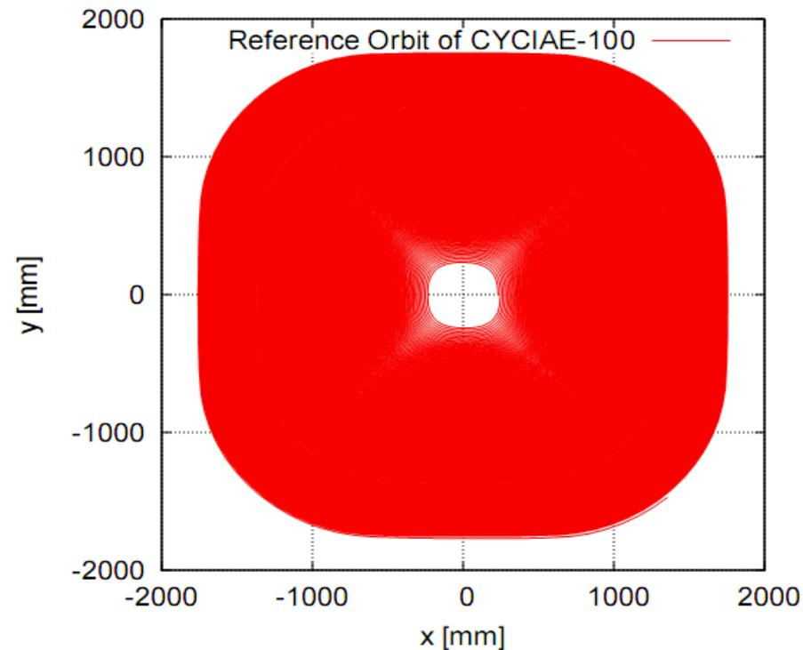
Calculation of the accelerating reference orbit of CYCIAE-100
