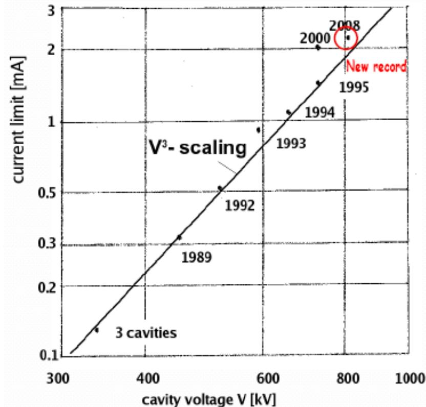
Space charge limits in PSI Ring cyclotron (courtesy by W.Joho, 1981)
