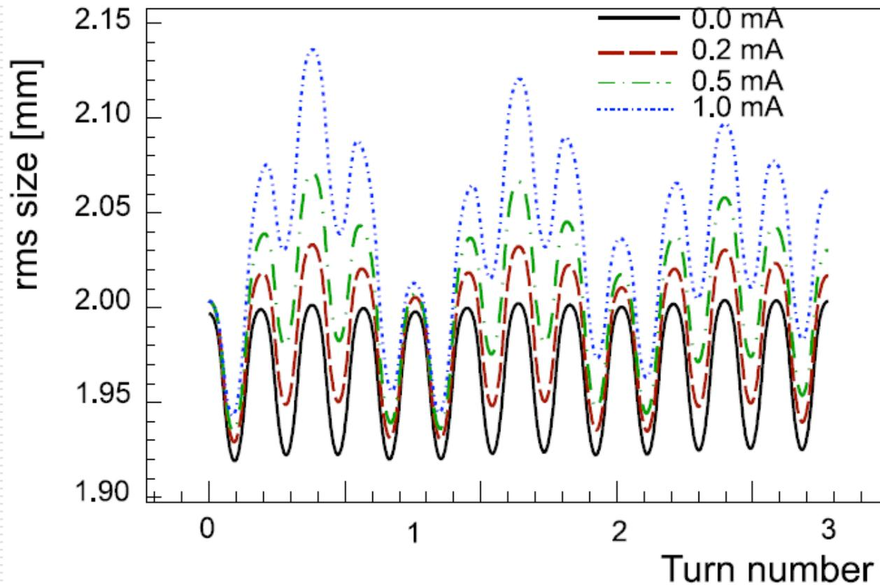
Mismatching in radial direction caused by space charge
