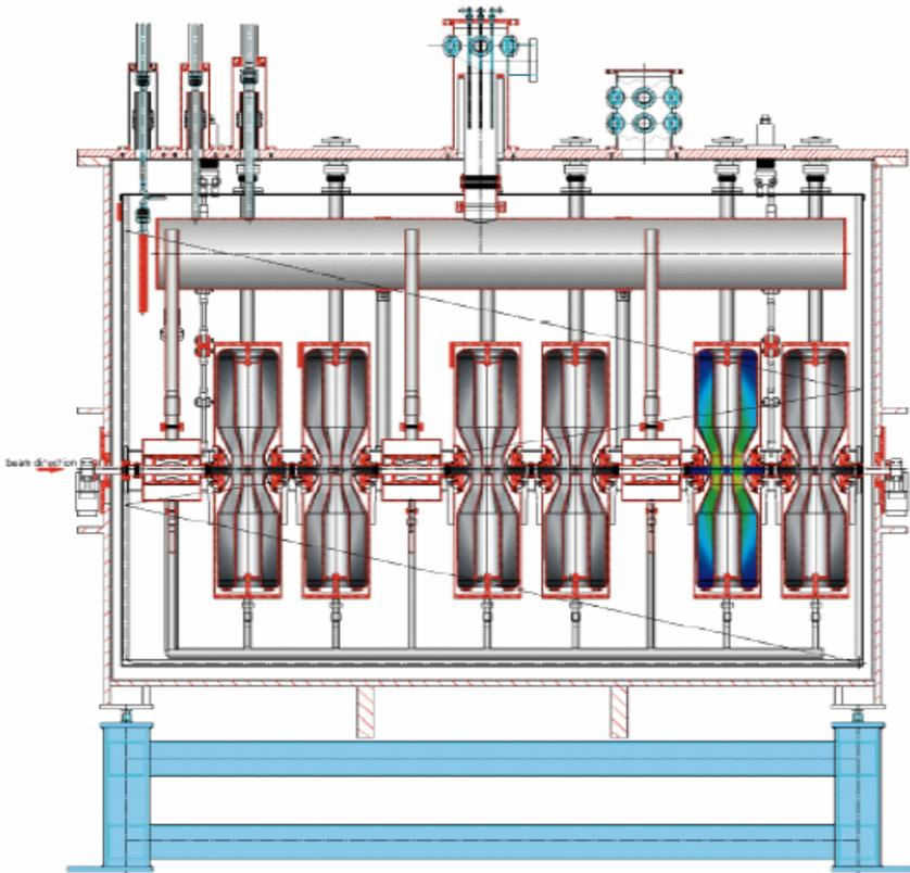
Prototype superconducting module with separate cavity and cryogenic vacuum. Fabrication by ACCEL
