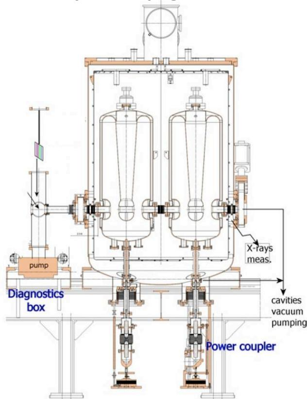
$\beta=0.12$  quarter-wave cryomodule
