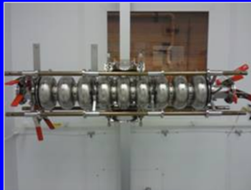
Cavity assembly rail, shown in vertical & horizontal orientation
