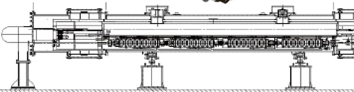
Four 9-cell cavities in the STF tunnel
