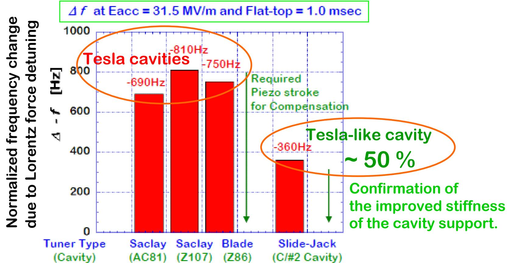
Required piezo stroke for compensation at 31.5 MV/m in Tesla-like cavity was reduced ~50 % of that in the Tesla cavities.
