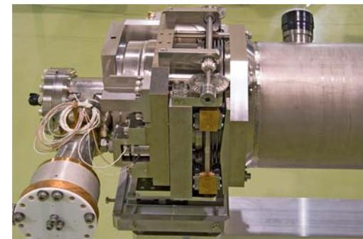
Slide-jack tuner and Piezo tuner
