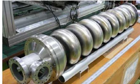
A niobium 9-cell cavity covered with Ti jacket
