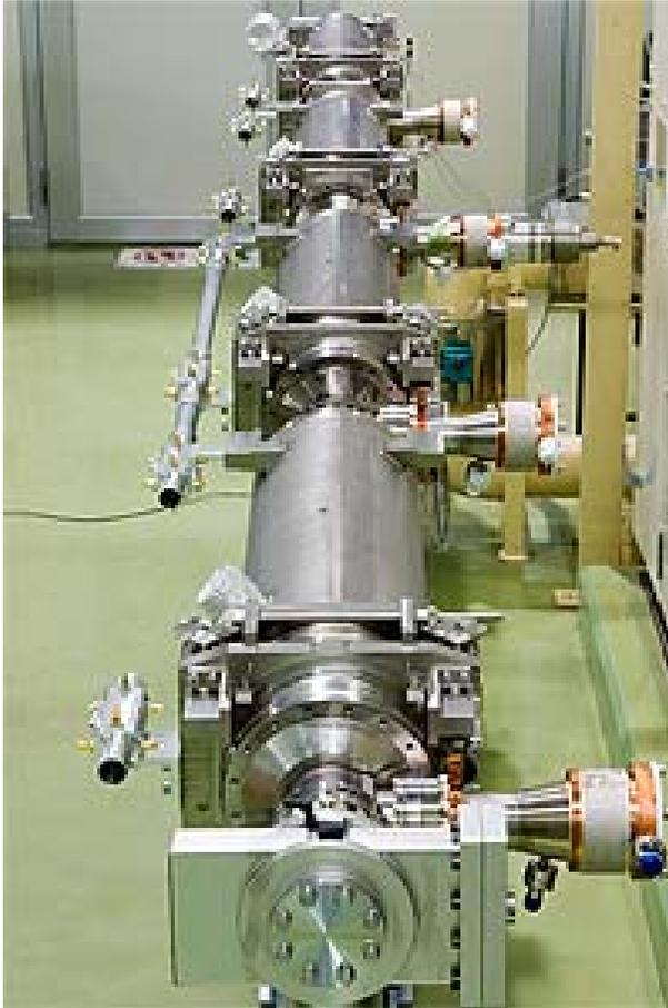
Tuner installation and alignment of four cavities at outside area of a clean room
