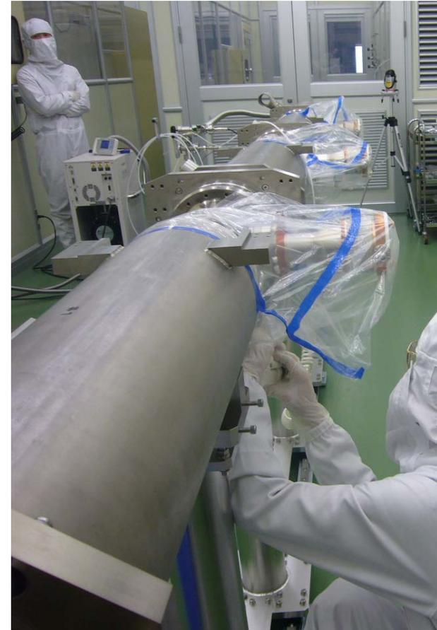
Vacuum leak-check of string cavities
