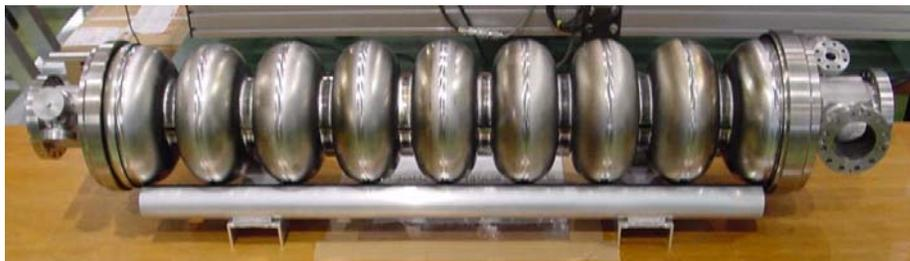
A Tesla-like 9-cell cavity with stiff Ti endplates
