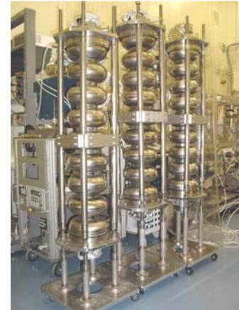
4 cavities in vertical tests
