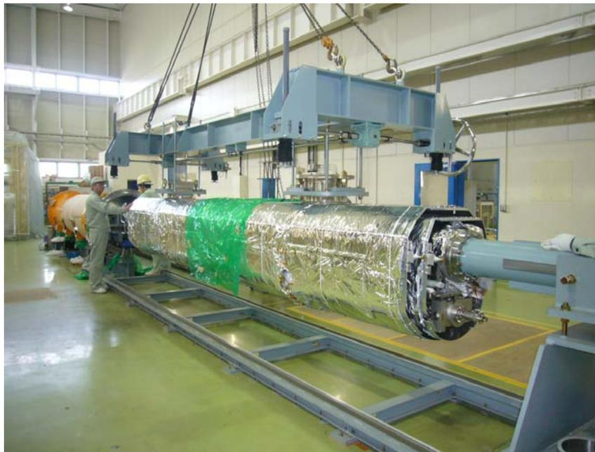
Insertion of an assembled cold mass into a vacuum vessel
