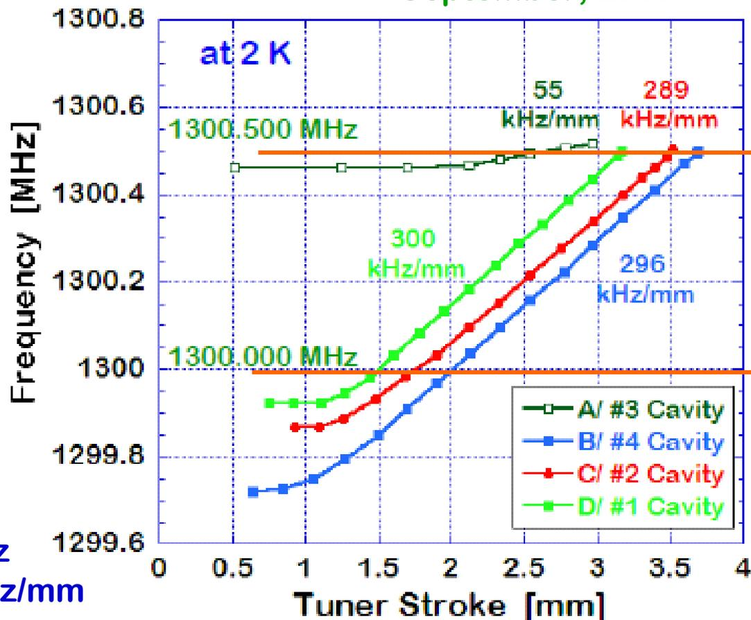
One cavity showed a strange performance due to mistake in the pre-tuning, so that an operating frequency changed to 1300.50 MHz to drive 4 cavities.
