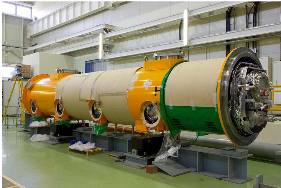
Completed STF cryomodule containing four Tesla-like cavities
