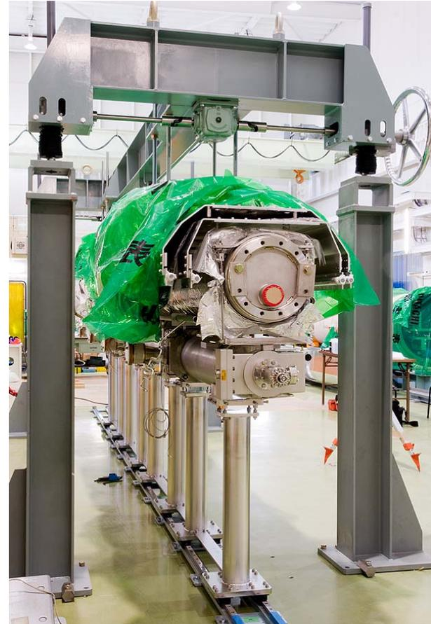
Hanging the string cavities on GRP at cryomodule assembly area
