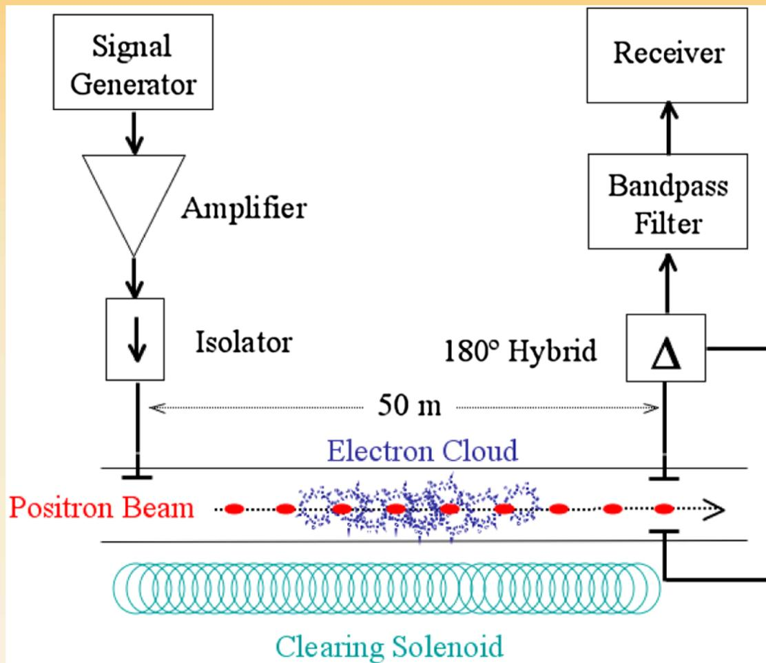
PEP II has the big advantage of a **50 meter long drift space where the electron cloud can be turned ON and OFF** by just powering a long solenoid to create a field of about 20 Gauss
