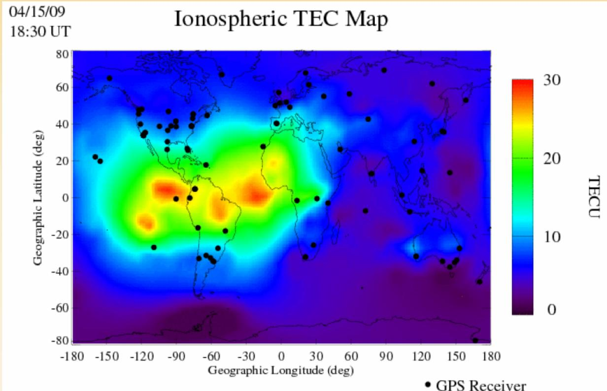
TEC is defined as the number of free electrons along the ray path above one square meter on the ionosphere and its unit is represented as TECU (1 TECU =  $10^{16}$  e<sup>-</sup>/m<sup>2</sup>)
