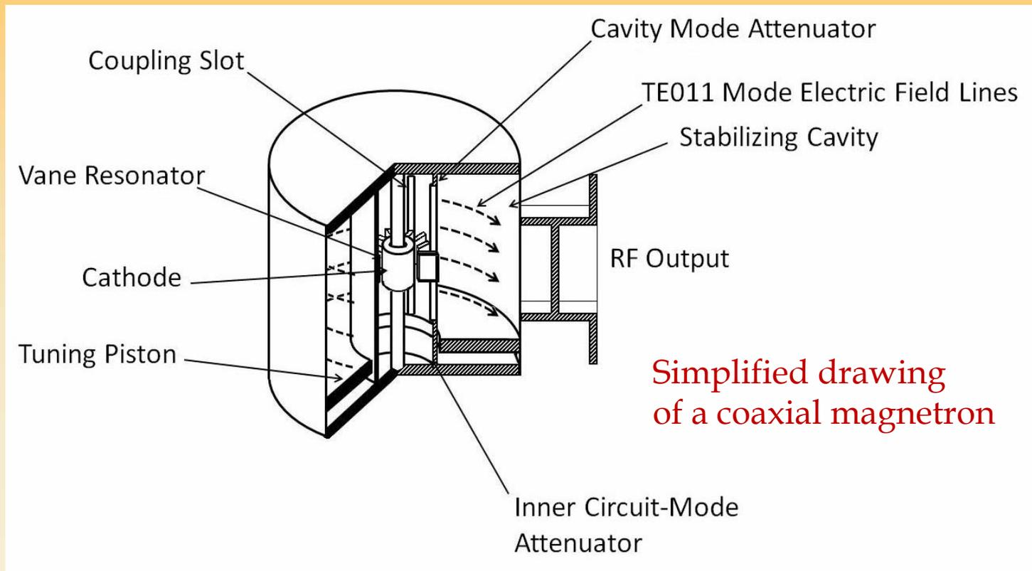
analogy between coupling slots in this structure and slots in LHC beam-screen ; for the LHC case the anode and cathode would be inverted since electrons come via photoeffect or secondary emission from inner surface of the beam-screen
