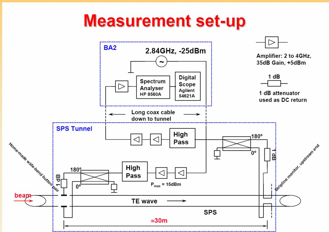
This first setup had a conventional spectrum analyzer with a digital scope connected to the (rear) IF output for time resolved signal acquisition
