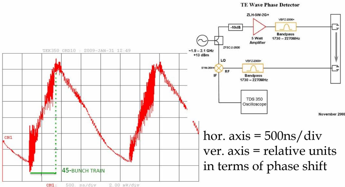
Phase shift dependence on beam current suggest electrons might reach higher densities near the beam pipe walls. That would be in good agreement with lower  $\Delta\phi$  measured.
