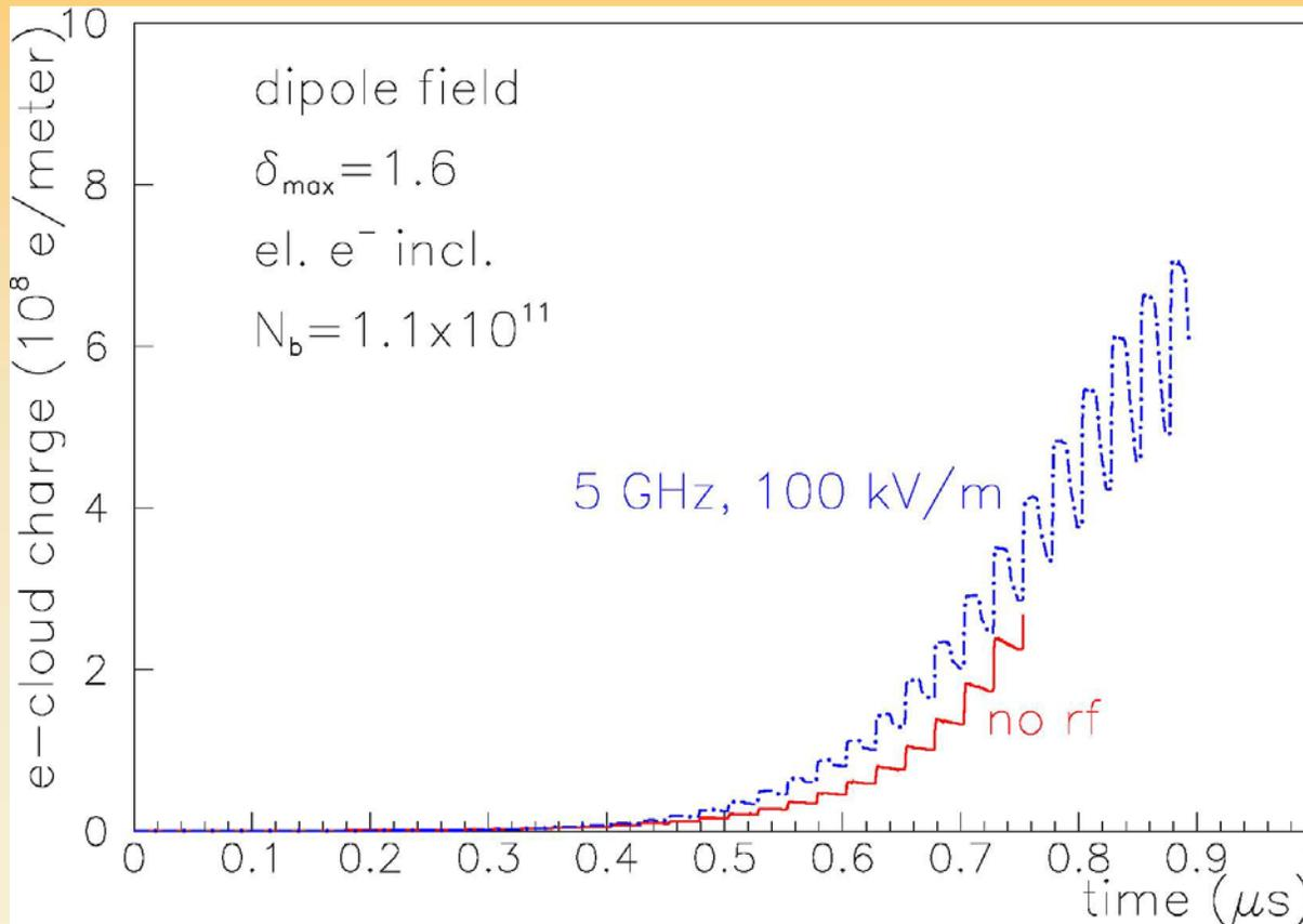
Simulation of electron-cloud build up in LHC dipole chamber with 2-cm radius with and without additional 5-GHz  $TE$ -mode microwave of amplitude 100 kV/m. **We notice a degradation with additional RF power**
