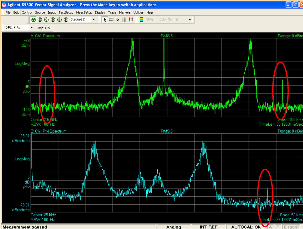
Applying the demodulation function we can clearly see the **AM contamination**
