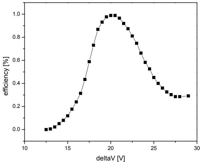
Efficiency for the production of  $\text{Cs}^{17+}$  as function of the potential difference between the singly charged ion source and the charge breeder
