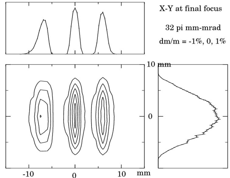
ion optical simulation for mass resolution after charge state breeding
