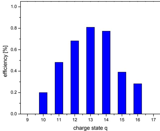
Efficiency for the production of high charge states of  $^{80}\text{Rb}$
