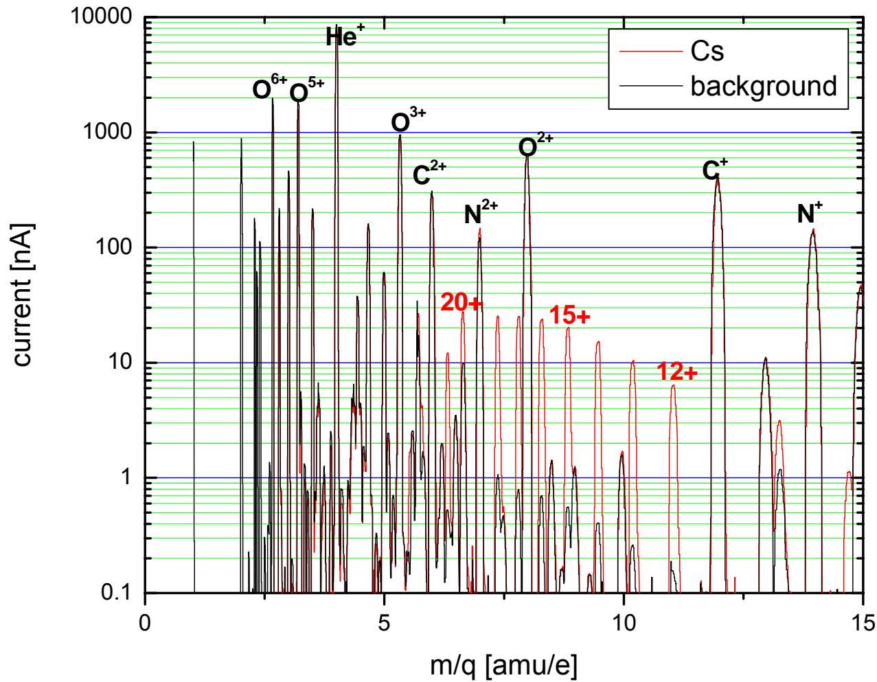
mass spectrum **with** and **without**  $\text{Cs}^+$  injection (500 W rf power)
