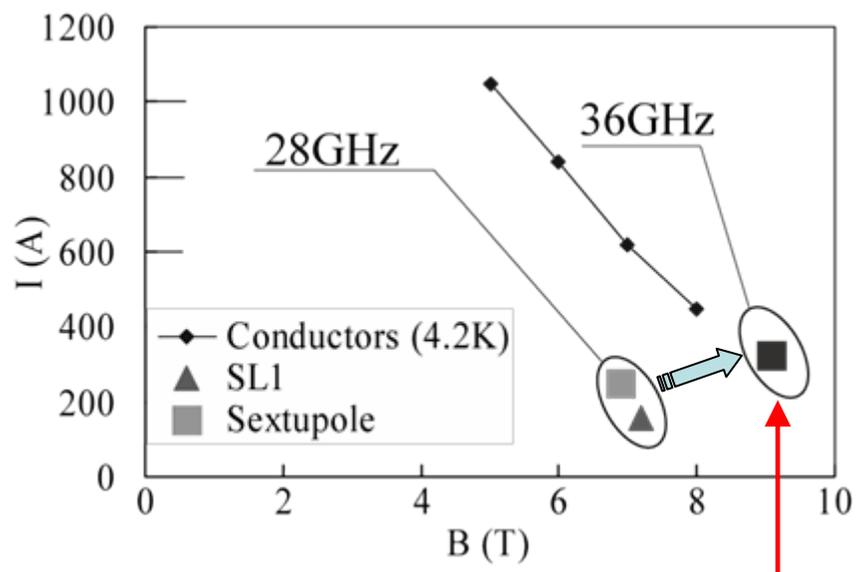
Exceed the critical current of NbTi wire at 4.2K
