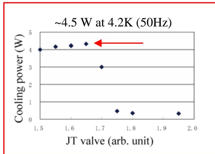
2 GM-JT refrigerator is installed for Cooling the SC-Coils of RIKEN SC-ECRIS
