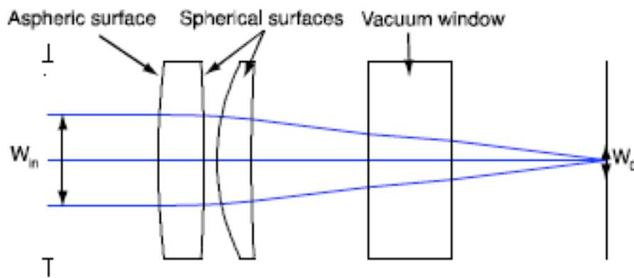
The  $W_{in}$  is the transverse laser beam radius and the  $W_0$  is the minimal spot size at the focus
