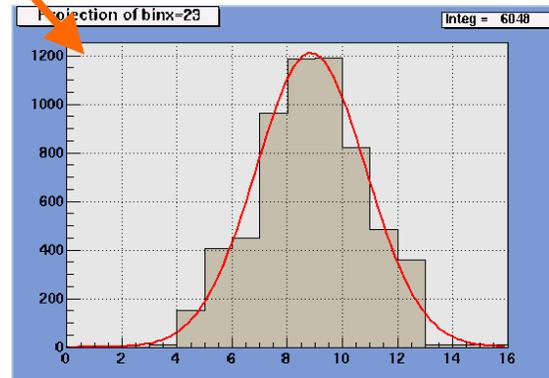
← Beam profile cross-section with Gaussian fit
