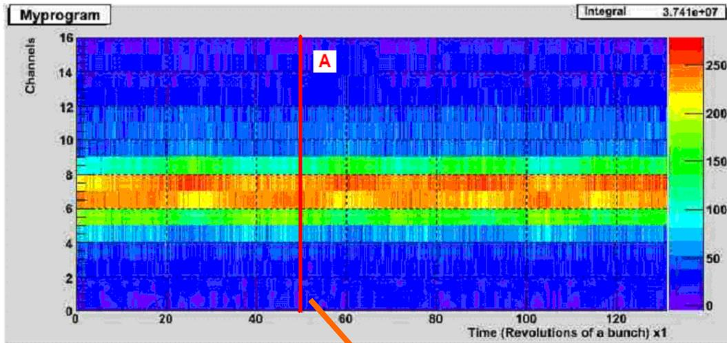
← Beam profile vs. the turn number. Colours indicate the particles intensity
