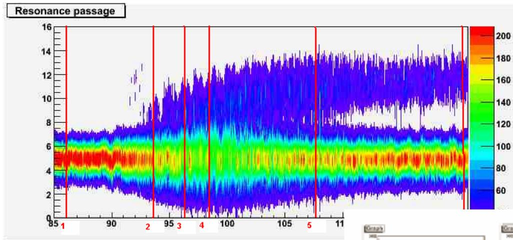
Time evolution of the vertical beam profile in the case of the particle trapping in the resonance island ( $\Delta t = 3s$ ).
