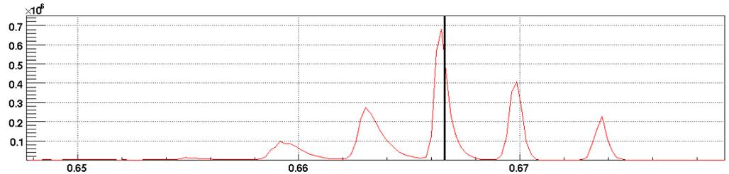
For high chromaticity the synchrobetatron resonances are observed.
