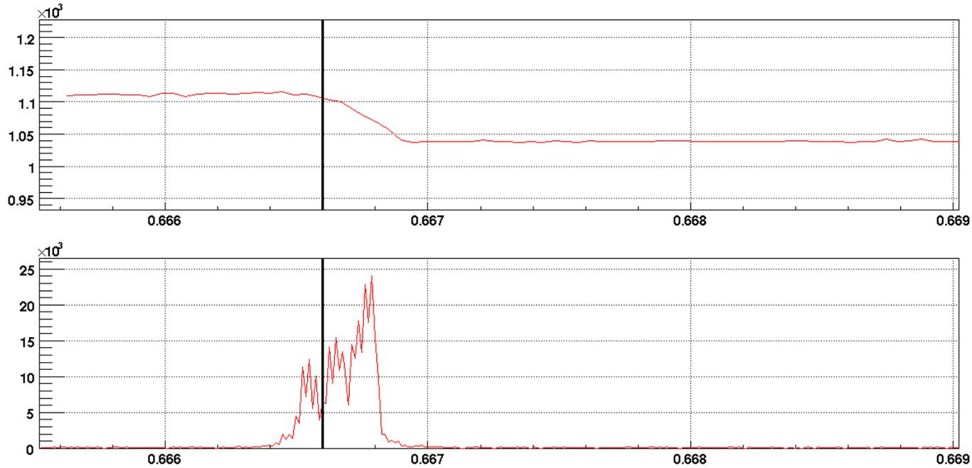
Total intensity decrease (upper plot) and particles loss rate (lower plot) during the resonance crossing. Tune change  $0.6687 \rightarrow 0.6653$  for 1 s,  $I = 0.212 \rightarrow 0.214$  mA
