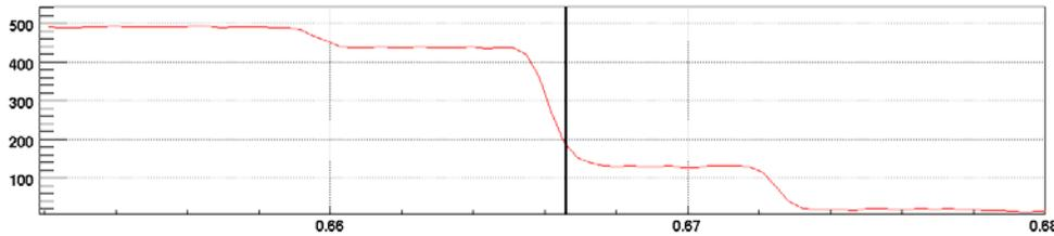
Particles loss while crossing the unstable resonance with synchrobetatron satellites
