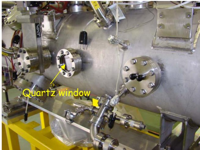
The quartz window was installed on the PETS tank to register the light emission during breakdown event.
