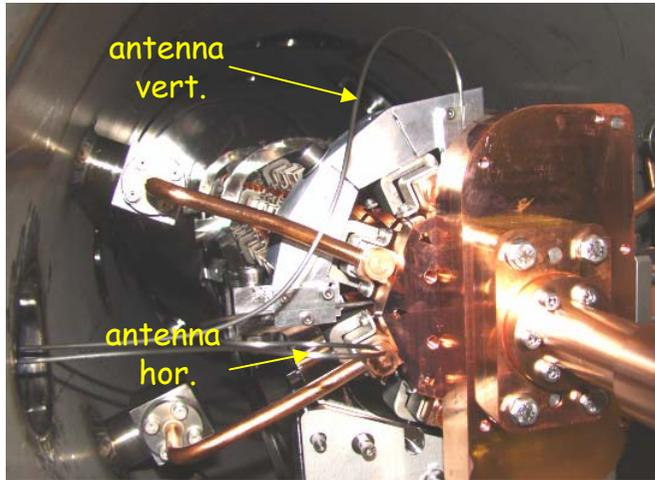
Two RF pick-ups were installed into the damping slots:
