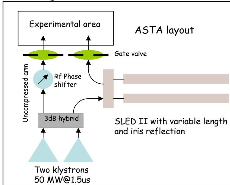
ASTA is a new generation general purpose test stand, which will allow processing the various types of the high power RF equipment at X-band. The facility can provide a very versatile pulse length and power level.
