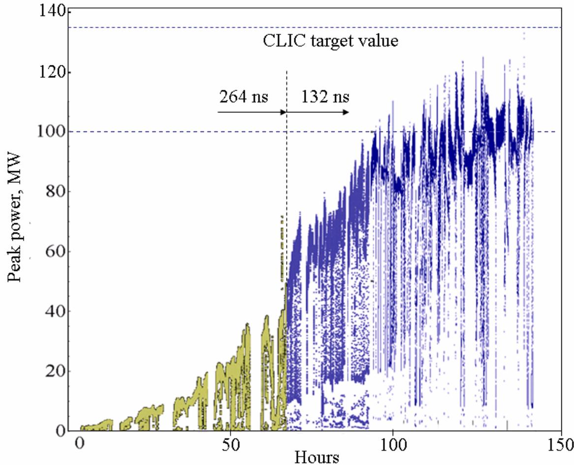
At a peak power level above 110 MW, the processing speed was practically saturated, mostly limited by vacuum interlocks on the ion pumps, especially after the breakdown event.
