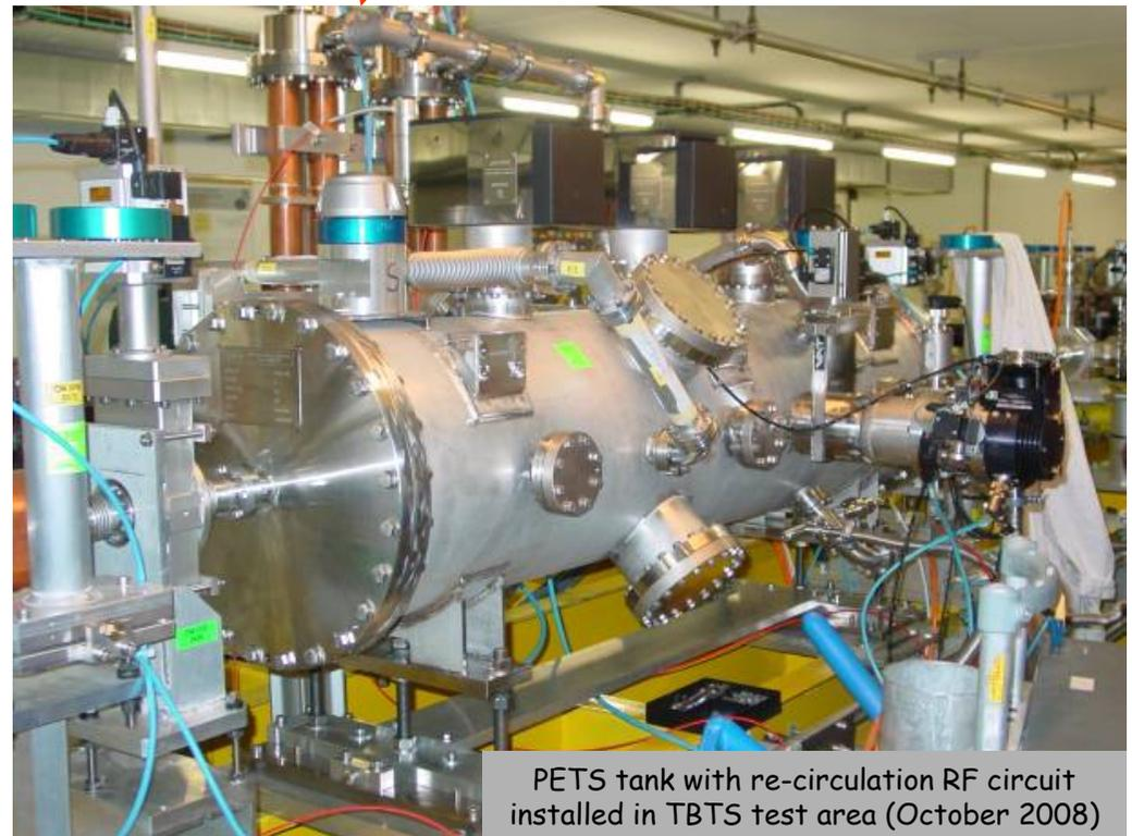
PETS tank with re-circulation RF circuit installed in TBTS test area (October 2008)
