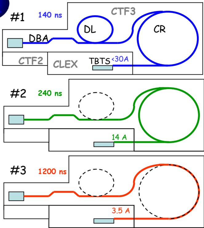
• To compensate for the lack of current, the active TBTS PETS length was significantly increased: from the original 0.215 m to 1 m.
