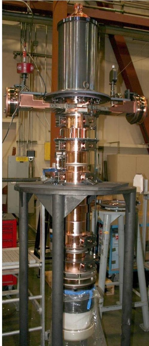
Klystron after exhaust
