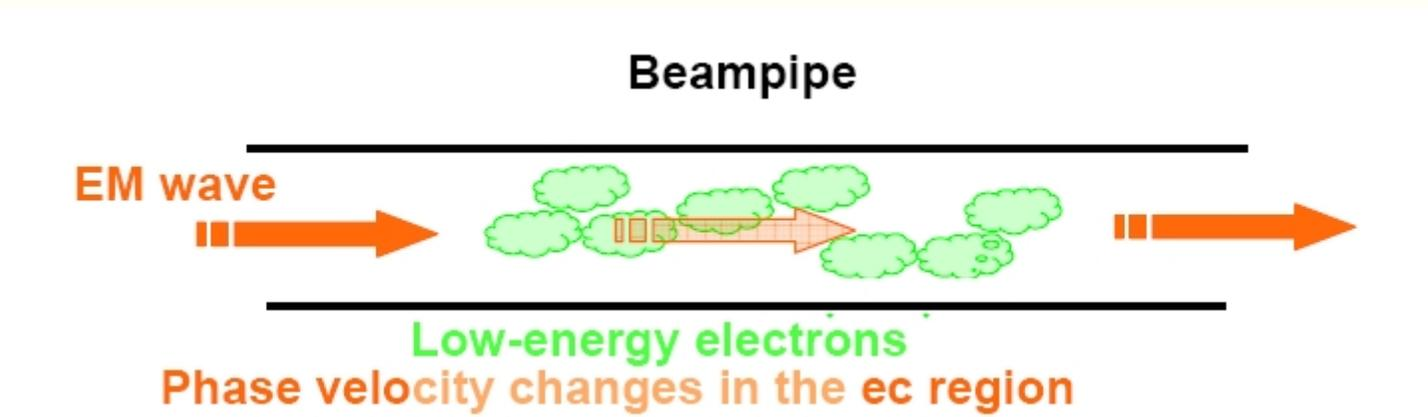
From plasma physics, expect a microwave travelling down a waveguide to experience a phase shift due to a homogeneous plasma
