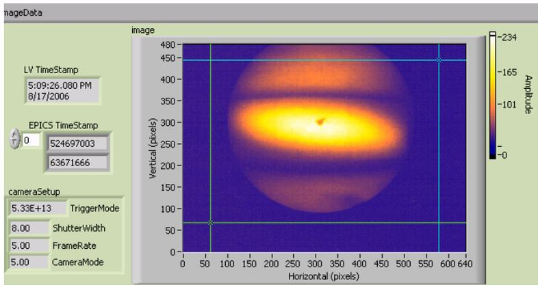
Tilted beam on the target view screen
