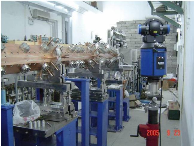
4 sections of the cavity were aligned with a laser tracker to reach an alignment accuracy of 30 $\mu$ m.
