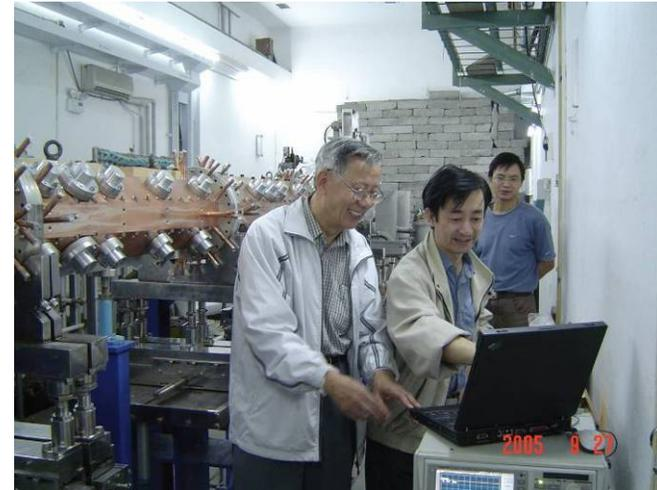
Bead-pull measurement for tuning the field with 64 movable Al tuners.
