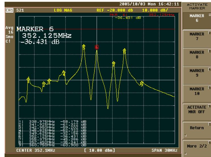
Spectrum of dipole modes are shifted by the dipole stabilizer rods.
