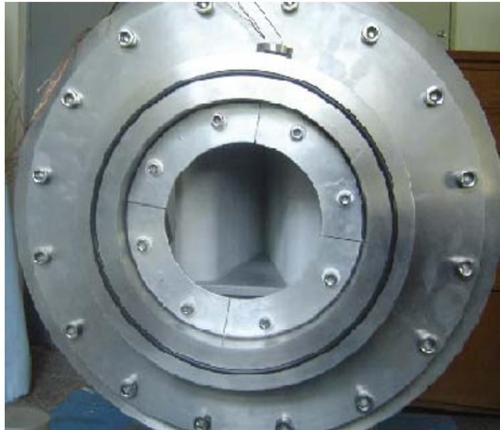
The new dumper with two slope plates
