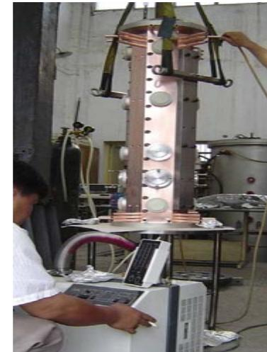
Vacuum leakage check
