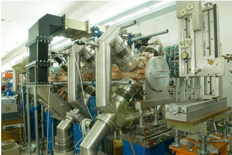
Bead pull measurement after the cavities are fully installed with all ports, except the end plates.
