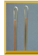
Absorber inside the 4th kicker chamber
