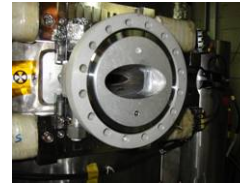
Pre-absorber in flange to protect the downstream bellows
