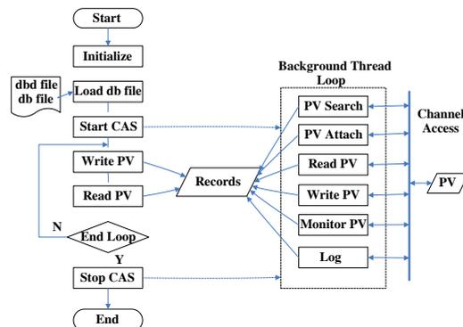
Figure 1: Flowchart of the LabVIEW PCAS Interface.
