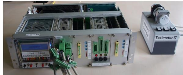
Figure 2: Newest version of ANKA-compact motor test system with display and stand-alone operator pulse control, which is used for direct verification of component compatibility to ANKA-Interface pinout, s. Figure 3. It is completed by power supplies for limit switches, encoder, two booster stages and a test stepper motor with limit/reference stop buttons and rotary encoder.
